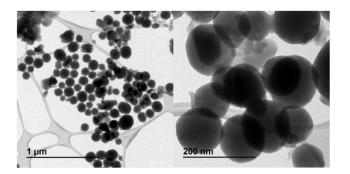
Fig. 2 SEM and TEM micrographs of POM-Chol-MSN as a representative sample.
