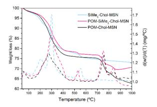
Fig. 1 TGA and DTA analysis curves for POM-Chol-MSN, POM-SiMe<sub>3</sub>-Chol-MSN, and SiMe<sub>3</sub>-Chol-MSN materials.
