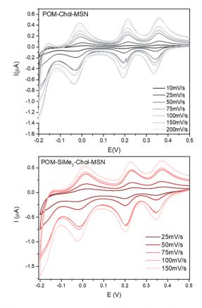
Fig. 9 Cyclic voltammograms of POM-SiMe $_3$ -Chol-MSN immobilized on a carbon-modified electrode as the working electrode in nitrogen saturated aqueous 0.5 M  $H_2SO_4$  vs. an Ag/AgCl/KCl (3 M) reference electrode and a platinum rod as the counter electrode.
