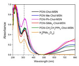
Fig. 4 DRUV-vis spectra of POM-based materials in comparison with that of H<sub>3</sub>[PMO<sub>12</sub>O<sub>40</sub>].
