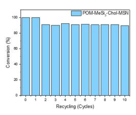
Fig. 14 The catalytic activity of POM-SiMe<sub>3</sub>-Chol-MSN in ten consecutive reaction cycles of oxidative desulfurization of DBT.
