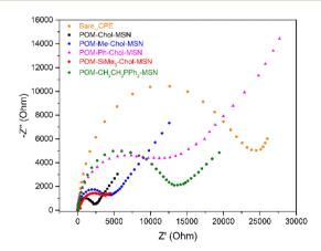
Fig. 11 Nyquist plots showing the modification of the materials recorded in 0.5 M  $H_2SO_4$  containing the redox system  $[Fe(CN)_6]^{3-/4-}$ .
