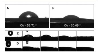
**Fig. 12** The contact angle of water on the surface of (A) SiMe<sub>3</sub>-Chol-MSN (B) Chol-MSN (C) POM-SiMe<sub>3</sub>-Chol-MSN and (D) the contact angle of the model oil in POM-SiMe<sub>3</sub>-Chol-MSN.
