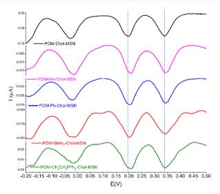
Fig. 10 Differential pulse voltammograms of polyoxometalate-based materials using a carbon-modified electrode as the working electrode in nitrogen saturated aqueous 0.5 M H<sub>2</sub>SO<sub>4</sub> vs. an Ag/AgCl/KCl (3 M) reference electrode and a platinum rod as the counter electrode.
