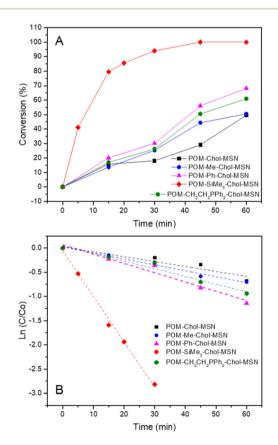
Fig. 13 The catalytic performance of POM based materials for DBT desulfurization. (A) Kinetic profiles and (B) pseudo-first order fit for different catalysts.
