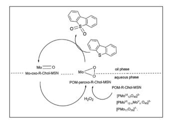
Fig. 17 The proposed mechanism for the oxidation of DBT by  $\rm H_2O_2$  catalyzed by POM-R-Chol-MSN in the model ion (two-phase) system.
