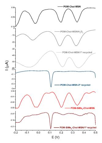
Fig. 15 DPV of POM-Chol-MSN and POM-SiMe $_3$ -Chol-MSN after two consecutive experiments immobilized on a carbon-modified electrode as the working electrode in nitrogen saturated aqueous 0.5 M  $H_2SO_4$  vs. an Ag/AgCl/KCl (3 M) reference electrode and a platinum rod as the counter electrode.
