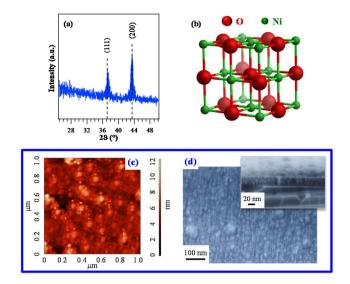
Fig. 6 (a) XRD pattern of a specimen grown on Si(100) from 3. The observed peaks can be assigned to cubic NiO (reference peak positions are marked), whose structure is reported in (b). Corresponding AFM (c) and plane-view FE-SEM images (d). In the latter case, a representative cross-sectional image is shown as the inset (film thickness  $\approx$  37 nm).
