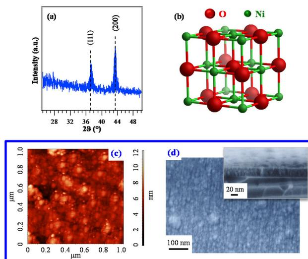
**Fig. 6** (a) XRD pattern of a specimen grown on Si(100) from 3. The observed peaks can be assigned to cubic NiO (reference peak positions<sup>70</sup> are marked), whose structure is reported in (b). Corresponding AFM (c) and plane-view FE-SEM images (d). In the latter case, a representative cross-sectional image is shown as the inset (film thickness  $\approx$  37 nm).
