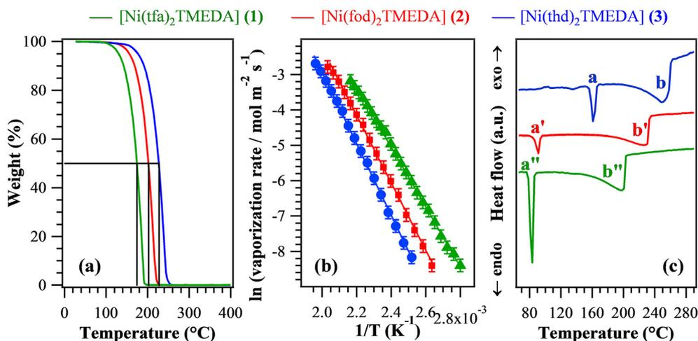
**Fig. 5** TGA curves (a), Arrhenius plot for the vaporization (b), and DSC traces (c) for compounds **1–3**. For the present compounds, in the investigated temperature interval, vaporization rate values ranged between  $2 \times 10^{-4}$  and  $8 \times 10^{-2}$  mol m<sup>-2</sup> s<sup>-1</sup>.
