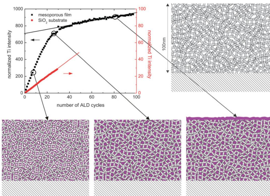
**Fig. 16** Normalized Ti XRF intensity as a function of the number of  $\text{TiO}_2$  ALD cycles on a planar  $\text{SiO}_2/\text{Si}$  substrate and on a mesoporous substrate with an initial average pore size of 4 nm. The cartoons display the gradual pore filling until completion followed by surface growth only. From Dendooven *et al.*<sup>161</sup>
