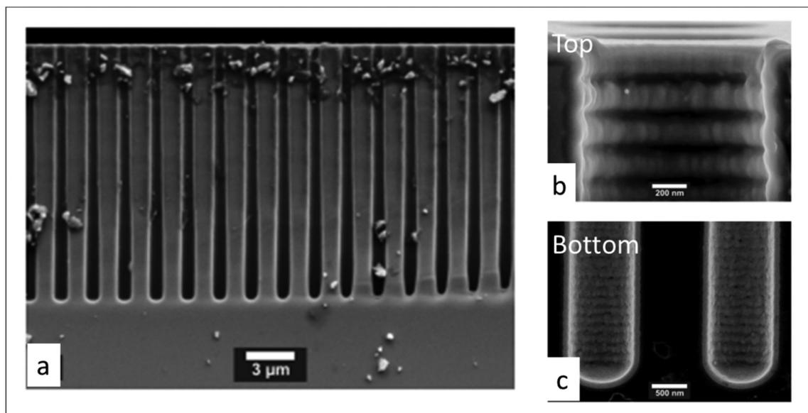
Fig. 14 Cross-sectional SEM images of 1  $\mu\text{m}$  diameter and 17  $\mu\text{m}$  deep pores array in silicon, conformally coated by atmospheric ALD of  $\text{Al}_2\text{O}_3$ . (a) Global structure, (b) pore opening and (c) pore bottom. From Poodt *et al.*<sup>153</sup>
