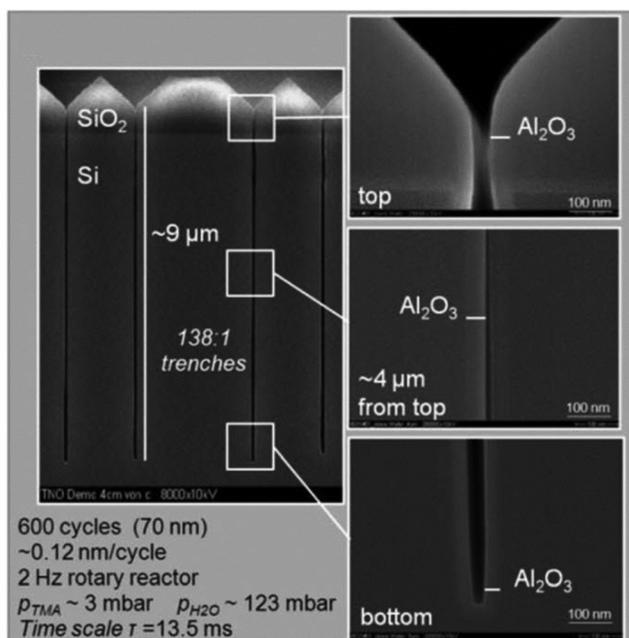
**Fig. 15** Cross-sectional SEM images of an  $\text{Al}_2\text{O}_3$  layer deposited at 1 atm. and  $200^\circ\text{C}$  in 138 : 1 aspect ratio trenches during 600 cycles in a rotary s-ALD reactor. (Trenched wafers kindly provided by Fraunhofer CNT/NamLab, Dresden). From Roozeboom *et al.*<sup>155</sup>
