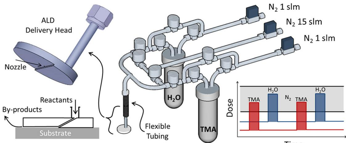
Fig. 7 Atmospheric t-ALD with a disk-shaped delivery head in an open-air environment. Reprinted with permission from Mousa et al.<sup>116</sup> Copyright 2015, American Chemical Society.
