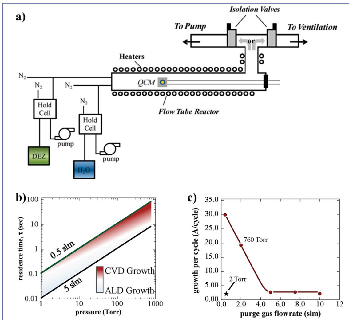
**Fig. 8** (a) Schematic of a flow tube ALD reactor (60 cm length and 3.8 cm inner diameter) design which allows for the deposition at pressures varying from vacuum to atmospheric, (b) residence time vs. operating pressure of the flow tube, and (c) GPC of ZnO at 760 and 2 Torr, using 30 s purge times vs. purge gas flow rate. Reprinted with permission from Jur *et al.*<sup>14</sup> Copyright 2011, American Chemical Society.
