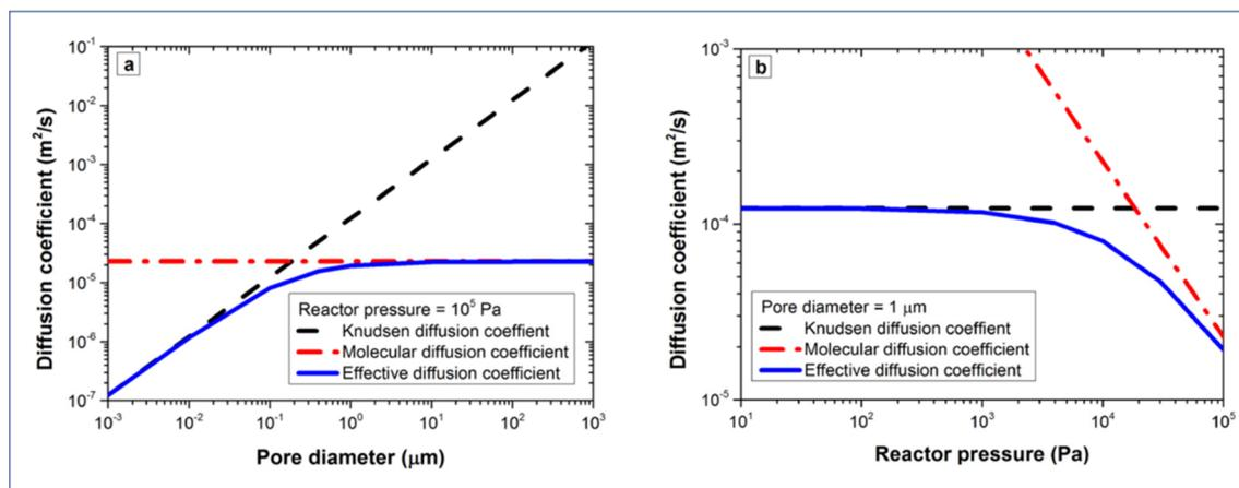
**Fig. 13** Diffusion coefficients of TMA as a function of (a) pore size at a fixed pressure of  $10^5$  Pa, and (b) reactor pressure for a fixed pore size of 1  $\mu\text{m}$ . From Poedt *et al.*<sup>153</sup>
