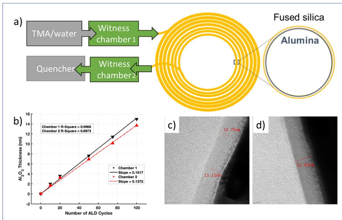
**Fig. 10** (a) Schematic overview of flow-through atmospheric t-ALD for the deposition of Al<sub>2</sub>O<sub>3</sub> on the capillary column, (b) measured Al<sub>2</sub>O<sub>3</sub> thickness grown on silicon in two different chambers after different numbers of ALD cycles, and TEM images of the respective film thickness at the entrance (c) and end (d) of the capillary column after 100 ALD cycles. From Patel *et al.*<sup>16</sup> Copyright 2022, American Chemical Society.
