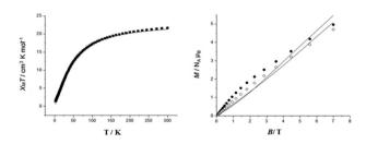
Fig. 6 (a) Temperature-dependent  $\chi_{\rm M}T$  of 8 in the temperature range 2 to 300 K (measured at 1000 Oe); the experimental data ( $\blacksquare$ ). (b) Field-dependent magnetization of 8 at 2 ( $\blacksquare$ ) and 4 K ( $\bigcirc$ ). Calculations for  $J=-5.2~{\rm cm}^{-1}$ , g=2.05 shown as full lines.
