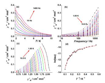
Fig. 10 Top, temperature dependence (a) and frequency dependence (b) of  $\chi''_{M}$  for complex 5 under a 0.4 T static field. Bottom, Argand plot (c) and fit of the  $ln(\tau)$  vs. inverse of temperature (d).
