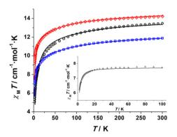
Fig. 7 Temperature dependence of the  $X_{\rm M}T$  product at 0.03 T for compounds 6 (squares), 7 (diamonds) and 8 (circles) (main curves). The  $\chi_{\rm M}T$  vs. T (100–2.0 K) variation for complex 5 is shown in the inset. Solid lines show the best fit of the experimental data.
