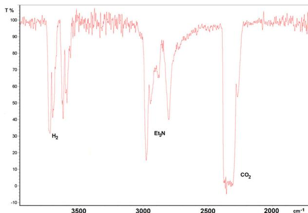
**Fig. 4** FTIR of the gas resulting from the solventless **3**-catalyzed (0.1 mol%) FADH in presence of Et<sub>3</sub>N at 353 K.
