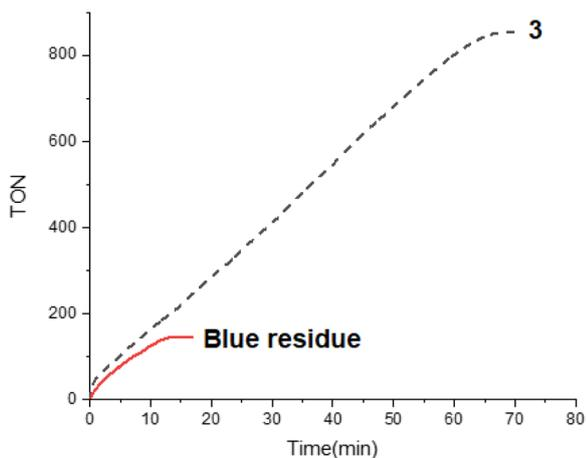
**Fig. 7** TON versus time (min) from the **3**-catalyzed (0.1 mol%) of FA (250  $\mu\text{L}$ ) in presence of  $\text{Et}_3\text{N}$  40 mol% or the blue-residue catalyzed solventless dehydrogenation of HCOOH (50  $\mu\text{L}$ ) at 353 K. The gas evolution was measured using a man on the moon<sup>TM</sup> reactor.<sup>22</sup>
