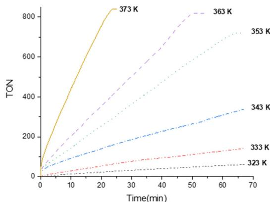
Fig. 3 TON versus time (min) from the **3**-catalyzed (0.1 mol%) solventless dehydrogenation of FA-Et<sub>3</sub>N adduct (Et<sub>3</sub>N 40 mol%) at different temperatures. The gas evolution was measured using a man on the moon™ reactor<sup>22</sup> (H<sub>2</sub>: CO<sub>2</sub> = 1 : 1).
