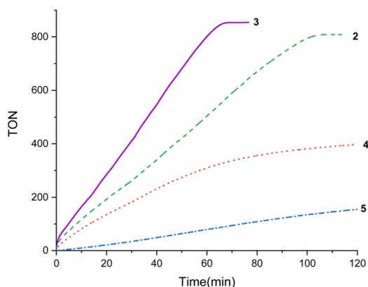
Fig. 2 TON versus time (min) from the **2**, **3**, **4** or **5** catalyzed (0.1 mol%) solventless dehydrogenation of FA-Et<sub>3</sub>N adduct (Et<sub>3</sub>N 40 mol%) at 353 K. The gas evolution was measured using a man on the moon™ reactor<sup>22</sup> (H<sub>2</sub>: CO<sub>2</sub> = 1 : 1).
