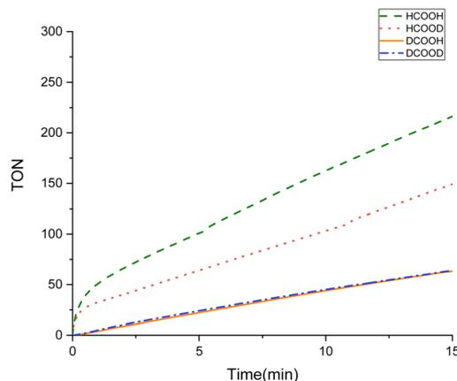
**Fig. 5** TON versus time (min) from the **3**-catalyzed (0.1 mol%) solventless dehydrogenation of HCOOH, HCOOD, DCOOH and DCOOD in presence of Et<sub>3</sub>N 40 mol% at 353 K. The gas evolution was measured using a man on the moon<sup>TM</sup> reactor.<sup>22</sup>
