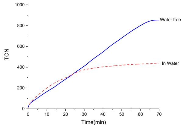
**Fig. 8** TON versus time (min) from the solventless **3**-catalyzed (0.1 mol%) of FA (250  $\mu\text{L}$ ) in presence of  $\text{Et}_3\text{N}$  40 mol% (blue) at 353 K or **3**-catalyzed (0.1 mol%) of FA (250  $\mu\text{L}$ )/ $\text{H}_2\text{O}$  (250  $\mu\text{L}$ ) in presence of  $\text{Et}_3\text{N}$  40 mol% at 353 K. The gas evolution was measured using a man on the moon<sup>TM</sup> reactor.<sup>22</sup>
