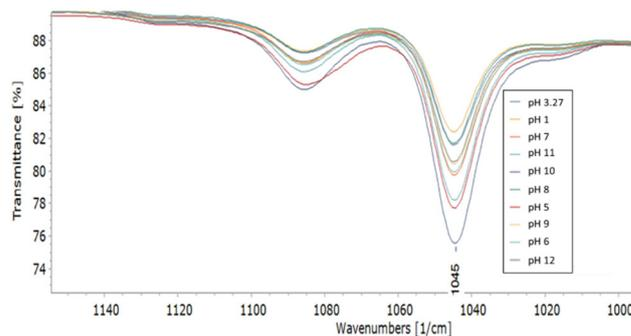
Fig. 4 IR spectra of  $[\text{Fe}(\text{bipy})_3]^{2+}$  solutions (0.5 M) at pH 1–12.
