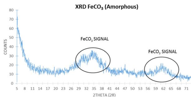
**Fig. 6** XRD pattern of  $\text{FeCO}_3$  precipitated during the carbonation reaction.
