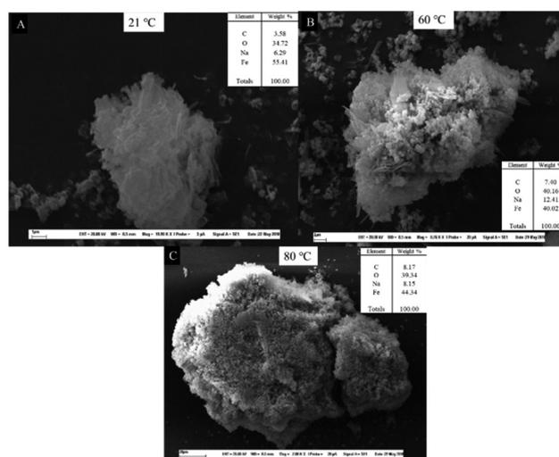
**Fig. 5** SEM images and EDS analysis (inset) of samples prepared at 21 °C (A) (19 980 $\times$ ), 60 °C (B) (8760 $\times$ ), and 80 °C (C) (2000 $\times$ ), using a polished section of the solid precipitate formed in the carbonation reaction.
