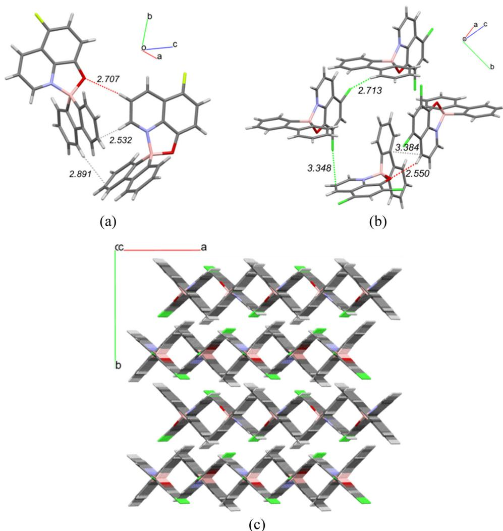
**Fig. 2** (a) CH $\cdots$ O and CH $\cdots$  $\pi$  hydrogen bonds inside the asymmetric unit of **3b**; (b) CH $\cdots$ O, CH $\cdots$ Cl, Cl $\cdots$  $\pi$ , and  $\pi\cdots\pi$  stacking between the adjacent molecules of complex **3d**; and (c) packing diagram of the crystal structure of complex **3d** along the *c* crystallographic axis.
