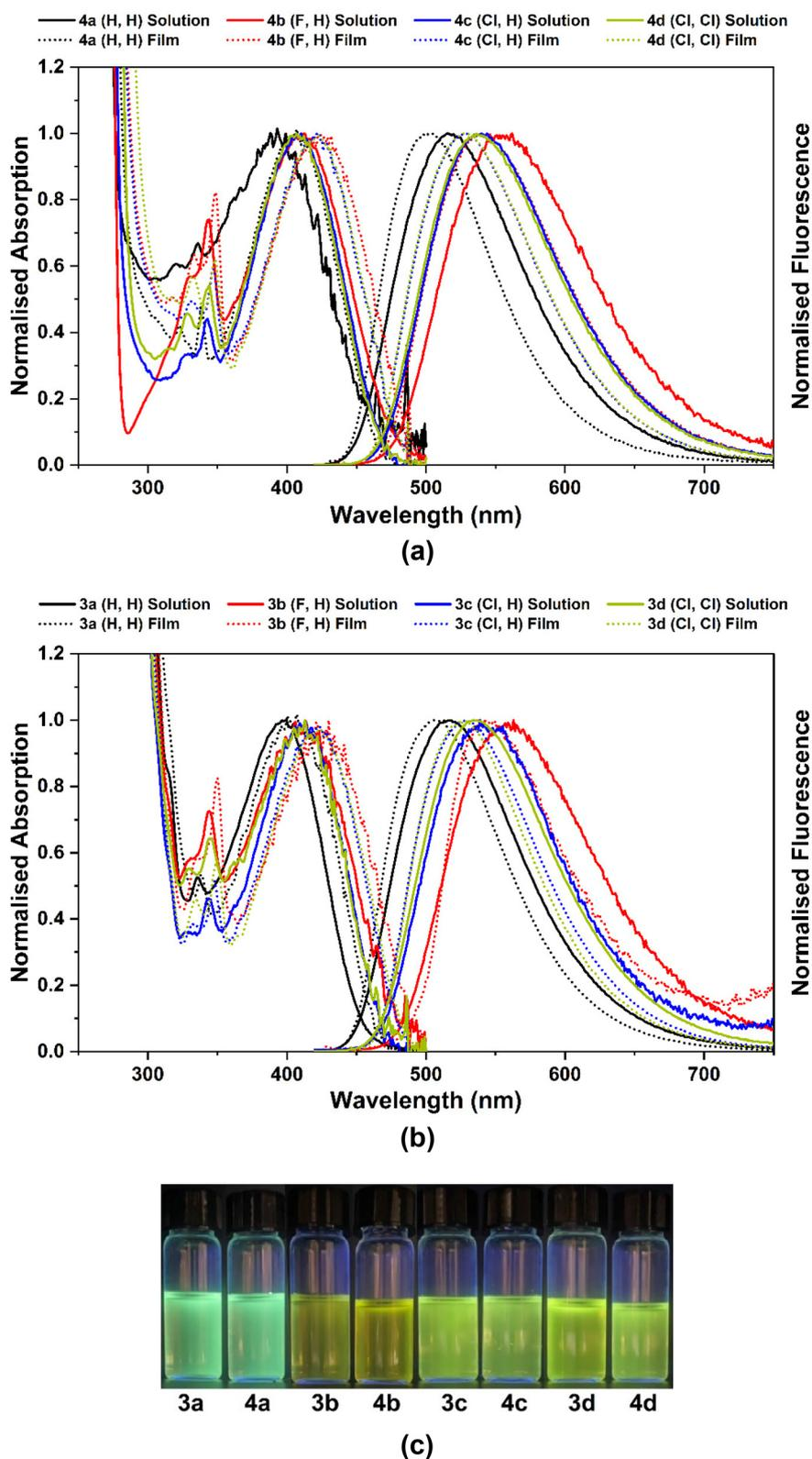
**Fig. 4** Normalised absorption and emission spectra of complexes: (a) 4a–d and (b) 3a–d in THF solution ( $OD_{\max} < 0.2$  at  $\lambda_{\text{abs}}^{\max}$ ;  $c < 8 \times 10^{-5}$  M) and in films (ZEONEX 480R, 1% wt), at 293 K. (c) Photoluminescence of the respective compounds in THF solution under 365 nm irradiation.
