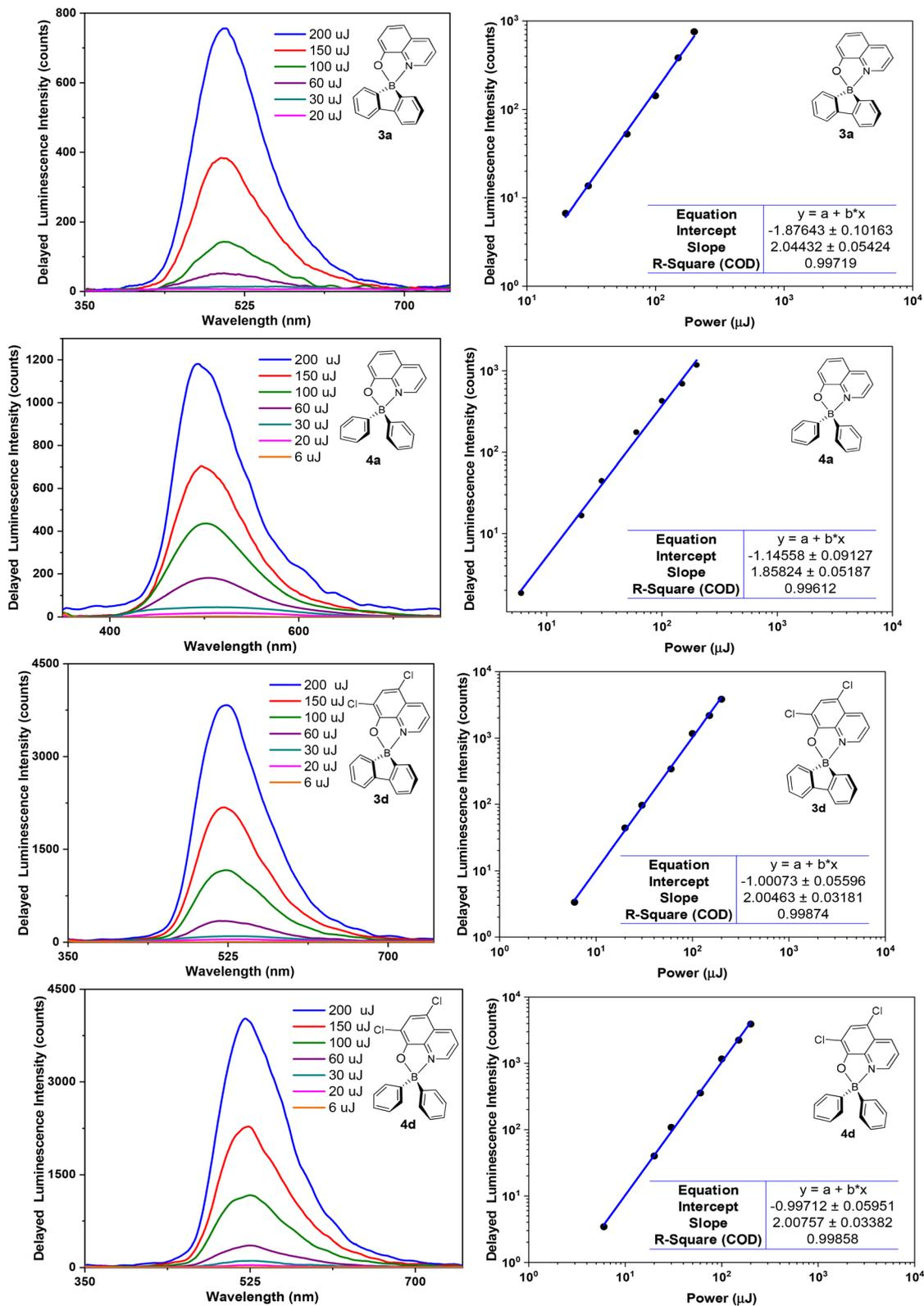
Fig. 7 Left: Dependence of DF intensity on the excitation dose for complexes **3a,d** and **4a,d** in ZEONEX 480R films at room temperature (ca. 293 K). Right: log–log plot of DF intensity as a function of excitation dose. A start delay (SD) of 20  $\mu$ s was used.
