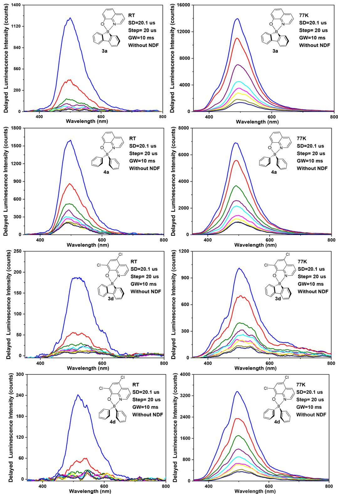
**Fig. 6** Transient emission spectra of complexes **3a,d** and **4a,d** in ZEONEX 480R films (1% wt) at room temperature (ca. 293 K) (left) and at 77 K (right). All spectra were recorded with a start delay (SD) of 20.1  $\mu$ s (blue curve) and with a delay increment of 20  $\mu$ s (step), with the use of a large gate width (GW = 10 ms). The delayed fluorescence intensity decreases at each delay increment.
