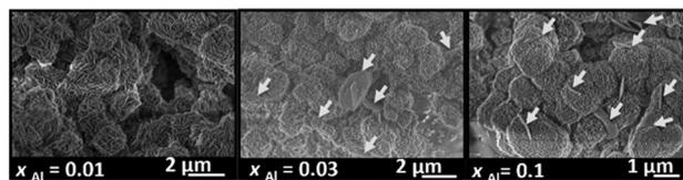
**Fig. 7** Morphology evolution in dependency of the aluminium content of the hydrozincite precursors. The arrows show the regions containing larger platelets and  $x_{\text{Al}}$  indicated the cation-based molar aluminium fraction.
