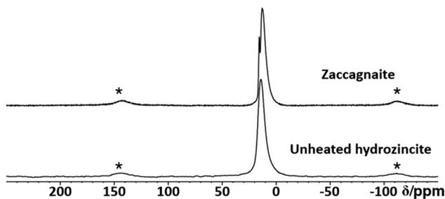
Fig. 8 Stack plot of  $^{27}\text{Al}$  MAS NMR spectra of a coprecipitated hydrozincite precursor with  $x_{\text{Al}} = 3\%$  aluminium incorporation and zaccagnaites. Spinning side bands are labelled with a star (\*).
