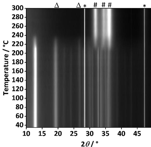
**Fig. 5** Temperature-resolved PXRD analysis of the thermal decomposition of the hydrozincite precursor containing 10% aluminium ( $x_{\text{Al}} = 0.1$ ). The PXRD analysis was performed with silicon as standard and in static air. The reflection positions are labelled as follows: silicon (\*), ZnO (#) and additional unassigned reflections ( $\Delta$ ).
