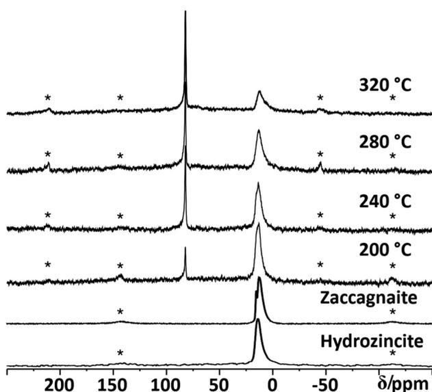
Fig. 12 Stack plot of  $^{27}\text{Al}$  MAS NMR spectra of the unheated hydrozincite, zaccagnaite and after being annealed at 200 °C, 240 °C, 280 °C and 320 °C for 4 h in static air with a heating ramp of 2 °C  $\text{min}^{-1}$  with  $x_{\text{Al}} = 0.005$  aluminium incorporation. All spectra were recorded with a spinning frequency of 20 kHz. Spinning side bands are signed with a star (\*).
