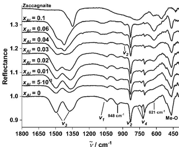
Fig. 9 Vibrational infrared spectroscopy of aluminium doped hydrozincites with different cation-based molar aluminium fractions  $x_{\text{Al}}$  in comparison with the aluminium rich zaccagnaites side phase  $\text{Zn}_4\text{Al}_2(\text{OH})_{12}(\text{CO}_3)\cdot 3\text{H}_2\text{O}$ .
