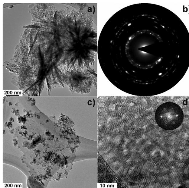
**Fig. 11** TEM-analysis of an aluminium doped zinc oxide sample (with  $x_{Al} = 0.03$ ). Image (a) visualizes a typical aggregate as it was also found by SEM. The corresponding electron diffraction pattern is shown in figure (b). The image in (c) shows a large single crystal with some fractions of the typical aggregate structure on top. A HRTEM micrograph of a part of that single crystal is shown in (d) with the corresponding FFT pattern.
