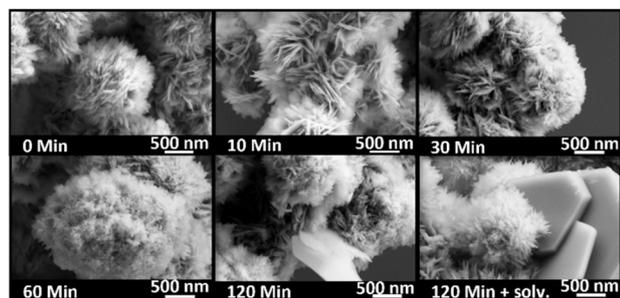
Fig. 2 SEM images depicting the morphology of the precursor materials recovered at different ageing times after co-precipitation at  $65^\circ\text{C}$  and a pH of 6.4 of a zinc–aluminium solution with an aluminium content of  $x_{\text{Al}} = 0.02$ .
