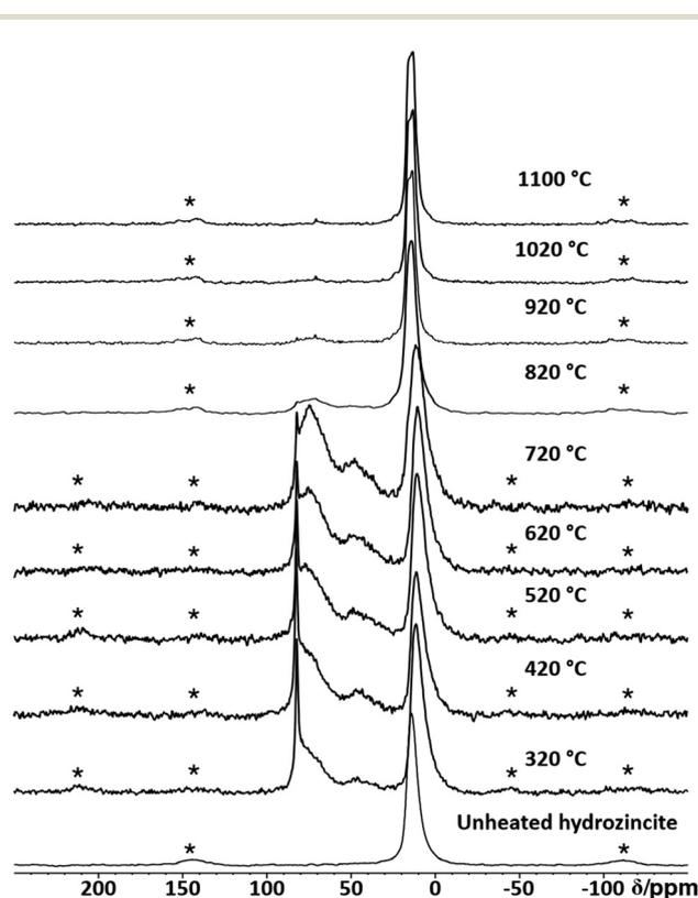
**Fig. 18** Stack plot of the  $^{27}\text{Al}$  MAS NMR spectra of aluminium doped zinc oxide with a cation-based molar aluminium fraction  $x_{\text{Al}} = 0.03$  after calcination at different temperatures. All spectra were recorded at a spinning frequency of  $20\text{ kHz}$ . Spinning side bands are labelled with a star (\*).
