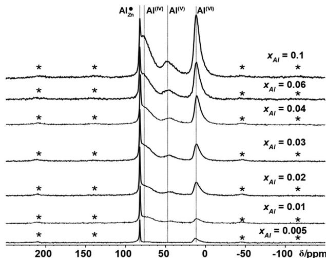
Fig. 13 Stack plot of  $^{27}\text{Al}$  MAS NMR spectra of zinc oxide, annealed with 320 °C for 4 h, with different cation-based molar aluminium fractions  $x_{\text{Al}}$ . All spectra were recorded with a spinning frequency of 20 kHz. Spinning side bands are signed with a star (\*).
