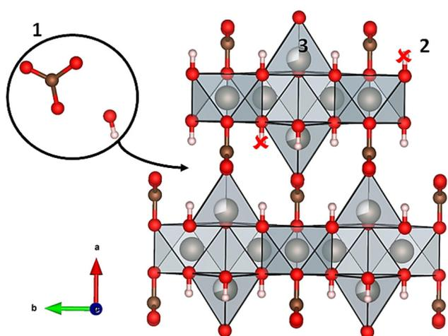
**Fig. 6** Schematic depiction of potential defects in hydrozincite for balancing the surplus positive charge resulting from substitution of  $\text{Zn}^{2+}$  by  $\text{Al}^{3+}$ : 1. Additional anions occupy the interlayer space. 2. Deprotonation of  $\text{OH}^-$  to form  $\text{O}^{2-}$  anions. 3. Vacancies on  $\text{Zn}^{2+}$  sites. The hydrogen atoms were placed at 0.9 Å distance and are not part of the crystal structure.<sup>43,48</sup>
