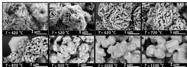
**Fig. 17** Morphology evolution depending on the calcination temperature of the undoped zinc oxide. Calcination was performed with  $2\text{ }^{\circ}\text{C min}^{-1}$  heating ramp and 4 h holding time in static air.
