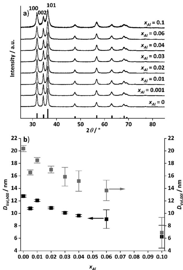
**Fig. 10** Powder XRD pattern of the aluminium doped zinc oxides (a) after calcination of the hydrozincite precursors at 320 °C with 2 °C min<sup>-1</sup> heating ramp and 4 h holding time in static air. The reference pattern (black bars) was taken from COD, zinc oxide (#2107059). (b) Sizes of the coherently scattering domains for the  $h00$  and  $00l$  reflections extracted via Pawley fit from the patterns shown in (a) as function of the cation-based molar aluminium fraction  $x_{Al}$ .
