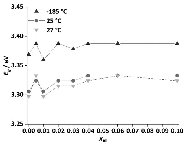
**Fig. 15** Band gap energies of the aluminium doped zinc oxides with different cation-based molar aluminium fraction  $x_{\text{Al}}$ . The measurements were performed at room temperature ( $25^\circ\text{C}$ , circles) at  $-185^\circ\text{C}$  (triangles) and at  $27^\circ\text{C}$  after cryogenic temperature measurement (upside down triangle). The measurements were performed under vacuum in transmission mode on a pellet containing dried KBr as diluent. The lines are to guide the eye.
