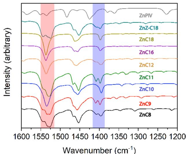
**Fig. 3** FTIR spectra of the zinc carboxylates, highlighting the  $\nu_s\text{ COO}$  ( $\sim 1540\text{--}1520\text{ cm}^{-1}$ ) highlighted in red and  $\nu_{as}\text{ COO}$  ( $1410\text{--}1395\text{ cm}^{-1}$ ) highlighted in blue.  $\Delta\nu$  for all samples is characteristic of bidentate ligands. The splitting of the resonances is indicative of asymmetric zinc centers.
