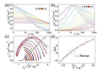
Fig. 5 Frequency dependence of the in-phase (a) and out-of-phase (b) ac susceptibility for complexes 3 under a 500 Oe dc field. (c) Cole–Cole plots at a dc field of 500 Oe for 3; the solid lines fit to the generalized Debye equation. (d) Magnetization relaxation time,  $\ln \tau vs. T^{-1}$  plot under a 500 Oe dc field. The red line represents the Raman fit relaxation process.
