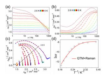
Fig. 4 Frequency dependence of the in-phase (a) and out-of-phase (b) ac susceptibility for complexes 2 under a 500 Oe dc field. (c) Cole–Cole plots at a dc field of 500 Oe for 2; the solid lines fit to the generalized Debye equation. (d) Magnetization relaxation time,  $\ln \tau vs. T^{-1}$  plot under a 500 Oe dc field. The red line represents the Raman and QTM fit relaxation processes.
