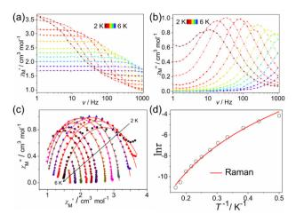
**Fig. 3** Frequency dependence of the in-phase (a) and out-of-phase (b) ac susceptibility for complexes **1** under a 500 Oe dc field. (c) Cole–Cole plots at a dc field of 500 Oe for **1**; the solid lines fit the generalized Debye equation. (d) Magnetization relaxation time,  $\ln \tau vs. T^{-1}$  plot under a 500 Oe dc field. The red line represents the Raman fit relaxation process.
