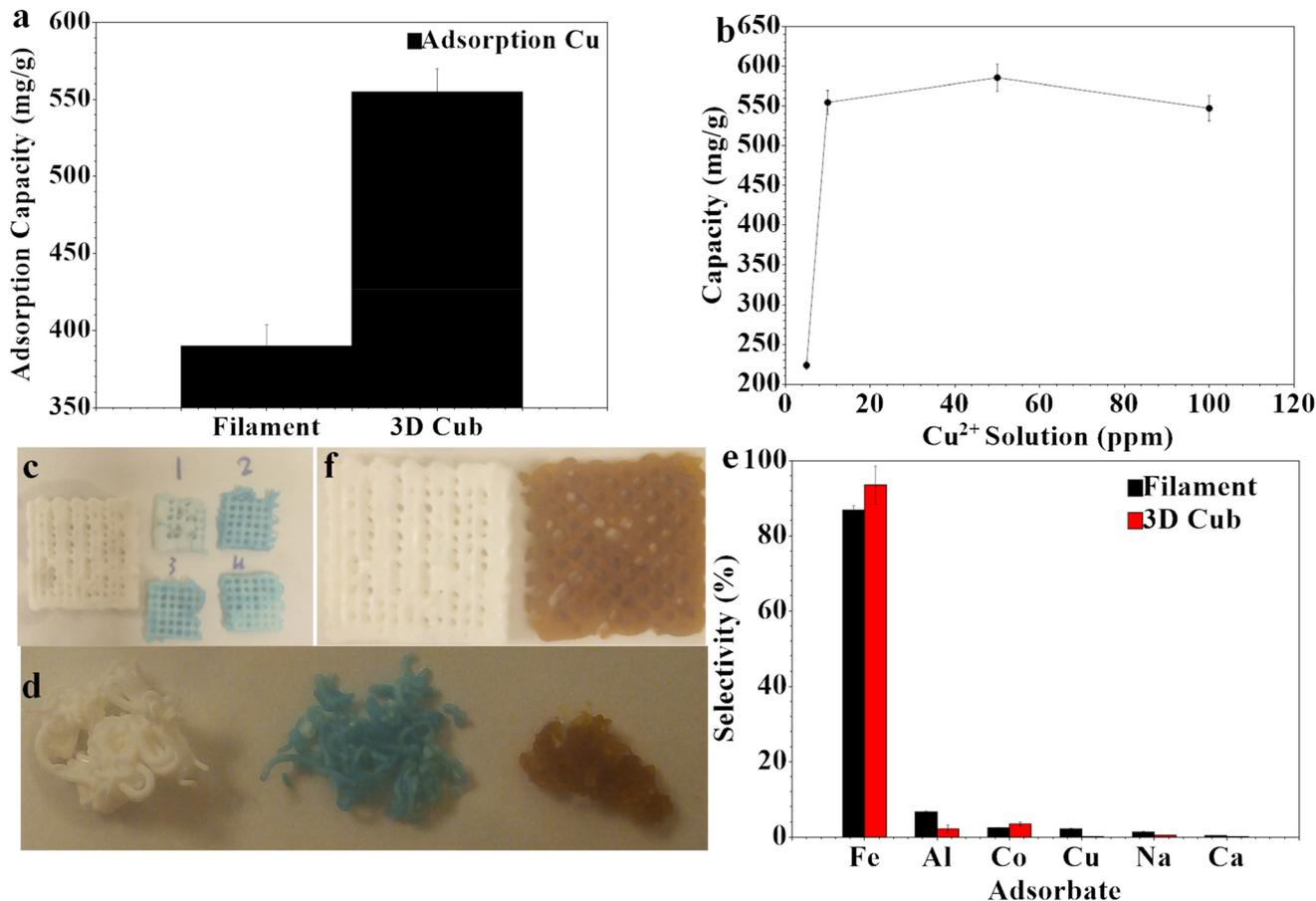
Fig. 7 (a) Adsorption capacity for Cu<sup>2+</sup> ions of the 3D cubes and filament, (b) adsorption of Cu<sup>2+</sup> ions using the 3D cubes with different initial concentrations, and (c) the cubes after adsorption of Cu<sup>2+</sup> at (1) 5 ppm, (2) 10 ppm, (3) 50 ppm and (4) 100 ppm, (d and f) objects after adsorption of mixed metal ions, and (e) selectivity toward different metal ions.
