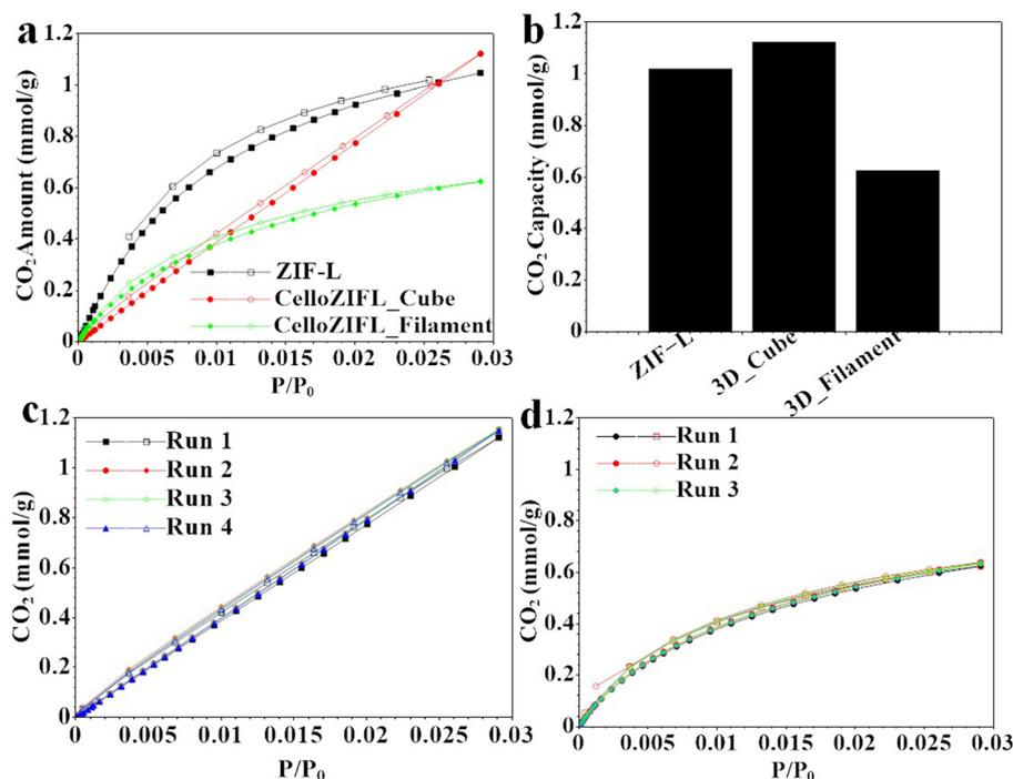
Fig. 6 (a) CO<sub>2</sub> adsorption–desorption isotherms, (b) CO<sub>2</sub> adsorption capacities, and (c and d) CO<sub>2</sub> recyclability of (c) 3D CelloZIF-L\_cubes and (d) 3D CelloZIF-L\_filament.
