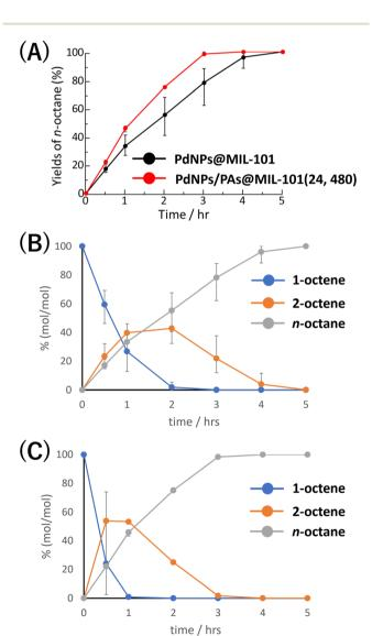
**Fig. 5** (A) Evolution of the hydrogenation of 1-octene with PdNPs@MIL-101 and PdNPs/PAs@MIL-101(24, 480) catalysts. (B) 2-octene and *n*-octane yields during the hydrogenation of 1-octene with the PdNPs@MIL-101 and (C) the PdNPs/PAs@MIL-101(24, 480) catalysts.
