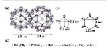
Fig. 1 Structures of (A) MIL-101 pores and (B) pore distances within clusters. (C) Proposed reaction to co-generate PdNPs and phosphate in the MOF structure.
