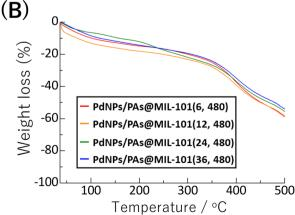
Fig. 2 (A) XRD data and (B) TG profiles of PdNPs/PAs@MIL-101(x, 480) (x = 6, 12, 24, 36).
