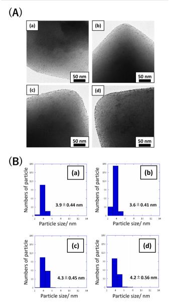
Fig. 3 (A) TEM images and (B) PdNP size distribution diagrams for PdNPs/PAs@MIL-101(x, 480): (a) x = 6, (b) x = 12, (c) x = 24, and (d) x = 36
