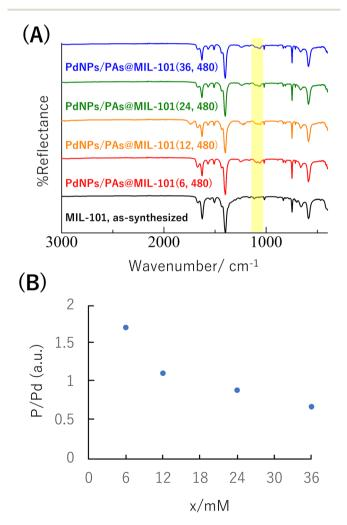
Fig. 4 (A) IR spectra of PdNPs/PAs@MIL-101(x, 480) (x = 6, 12, 24, 36). The peaks corresponding to P $\rightarrow$ O stretching vibration are highlighted in yellow. (B) P/Pd ratio in PdNPs/PAs@MIL-101(x, 480) (x = 6, 12, 24, 36).
