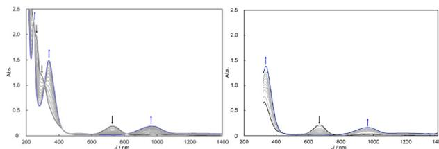
Fig. 2 Spectral changes of  $[\text{IV},\text{IV}_1\text{H}]^{3+}$  (0.13 mM) into  $[\text{III},\text{IV}_1\text{H}]^{2+}$  via the formation of  $[\text{IV},\text{IV}]^{2+}$  in dehydrated methanol (left) and those directly into  $[\text{III},\text{IV}_1\text{H}]^{2+}$  in acetone (right) under air at 25 °C.
