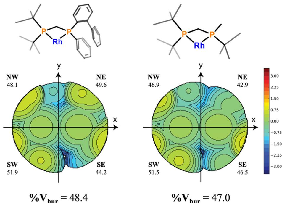
**Fig. 13** Topographic steric maps and  $\%V_{\text{bur}}$  values (for each quadrant and average value) of **BiphtBu** using the crystal structure of **RhBiphtBu** (Fig. 7) (left) and TCFP using the crystal structure of  $[\text{Rh}(\text{cod})_2\text{TCFP}]\text{BF}_4$ <sup>19</sup> (right).
