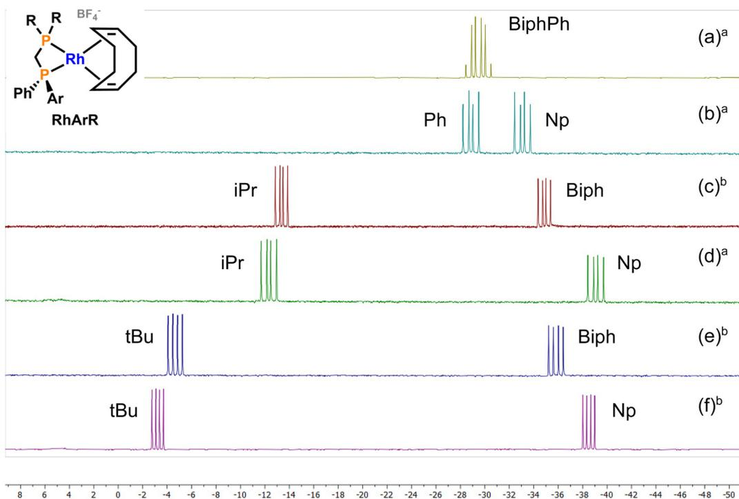
**Fig. 6** <sup>31</sup>P{<sup>1</sup>H} NMR (CD<sub>2</sub>Cl<sub>2</sub>) spectra of the mono(chelated) Rh complexes. (a) RhBiphPh, (b) RhNpPh, (c) RhBiphiPr, (d) RhNpiPr, (e) RhBiphtBu, (f) RhNptBu. <sup>a</sup> At 162 MHz. <sup>b</sup> At 202 MHz.
