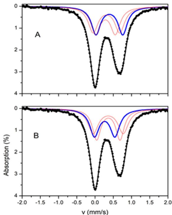
**Fig. 7** Mössbauer spectra from powdered samples of **2** at 295 K. The solid lines are simulations assuming two different models A and B as described in the text. The contribution of the three sites in the two models is included.
