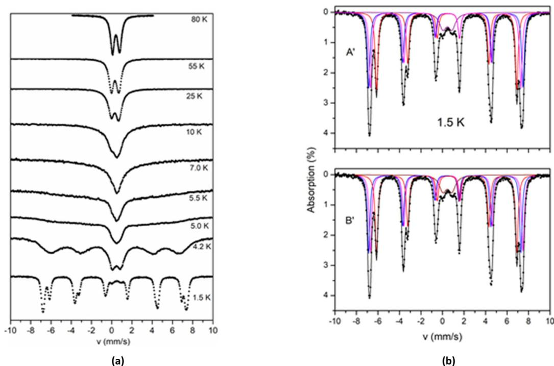
**Fig. 8** (a) Mössbauer spectra from a powder sample of **2** recorded at the indicated temperatures. The spectra are arbitrarily scaled in the y-axis. (b) The Mössbauer spectrum from a powder sample of **2** at 1.5 K. Solid lines are simulations assuming two different models A' and B' as described in the text. The contribution of the four sites in the two models is included.
