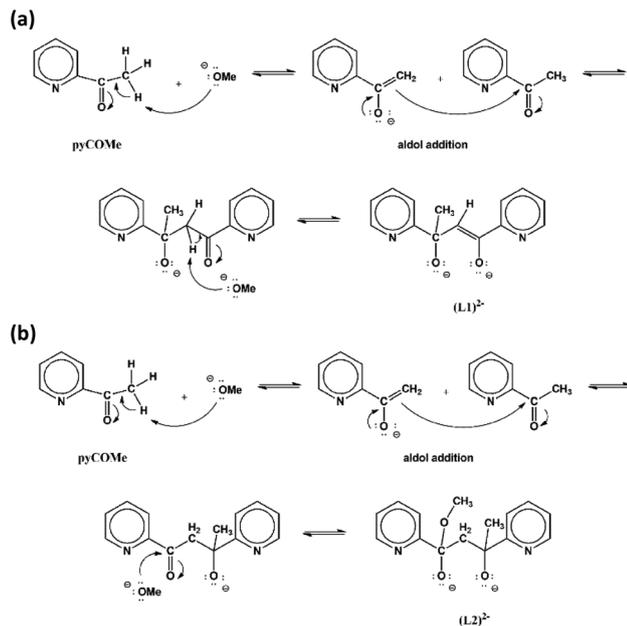
**Scheme 1** The proposed mechanisms for the formation of (L1)<sup>2-</sup> (a) and (L2)<sup>2-</sup> (b).
