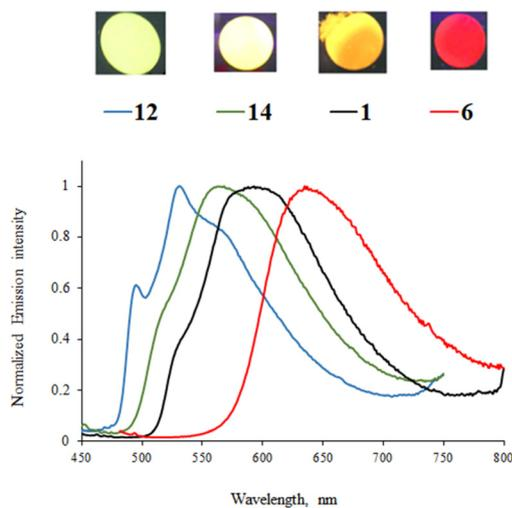
**Fig. 6** Solid state emission (2 wt% in the KBr matrix) of complexes **1**, **6**, **12**, and **14**.  $\lambda_{\text{exc}} = \lambda_{\text{max}}^{\text{abs}}$  of the lowest energy band in  $\text{CH}_2\text{Cl}_2$  solution. Inset: Pictures of the KBr pellets taken under UV irradiation (from left to right: **12**, **14**, **1**, and **6**).
