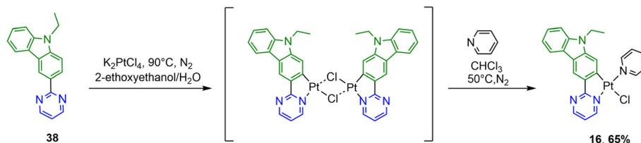
Scheme 2 Synthesis of N<sup>^</sup>C cyclometalated chloro-Pt(II) complex 16.
