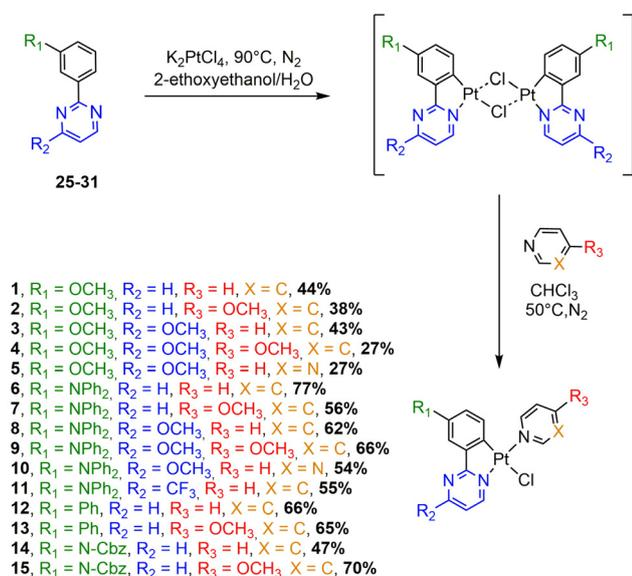
Scheme 1 Synthesis of N<sup>^</sup>C cyclometalated chloro-Pt(II) complexes 1–15.
