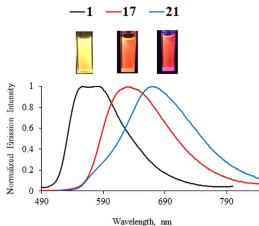
**Fig. 5** Normalized emission spectra of methoxy-substituted complexes **1**, **17**, and **21** in deoxygenated  $\text{CH}_2\text{Cl}_2$  solution ( $C \sim 10^{-5}$  M).  $\lambda_{\text{exc}} = \lambda_{\text{max}}^{\text{abs}}$  of the lowest energy band. Inset: Picture of the  $\text{CH}_2\text{Cl}_2$  solutions taken under UV irradiation (from left to right: **1**, **17**, and **21**).
