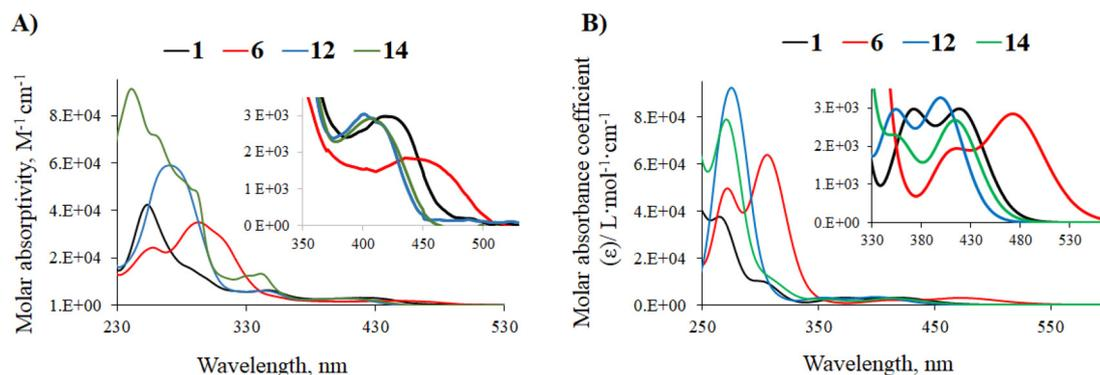
**Fig. 3** (A) UV-Vis absorption spectra of phenylpyrimidine complexes **1**, **6**, **12**, and **14** in  $\text{CH}_2\text{Cl}_2$  solution ( $C \sim 10^{-5}$  M). (B) TD-DFT-simulated UV-vis absorption spectra of complexes **1**, **6**, **12**, and **14**.
