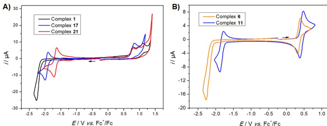
**Fig. 2** (A) Cyclic voltammograms of complexes **1** (black), **17** (blue), and **21** (red). (B) Cyclic voltammograms of complexes **6** (orange) and **11** (blue). CV obtained by using a Pt working electrode in 0.1 M  $\text{NBu}_4\text{PF}_6$  in  $\text{CH}_2\text{Cl}_2$  ( $E/V$  vs.  $\text{Fc}^+/\text{Fc}$ ,  $\nu = 0.1$   $\text{V s}^{-1}$ ,  $C = 0.5$  mM). The arrow indicates the scanning direction from the initial potential.
