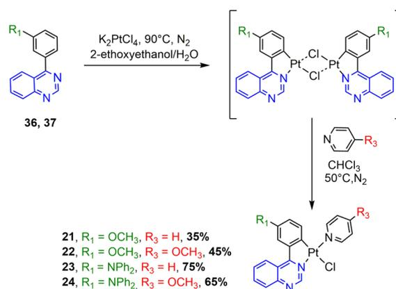
Scheme 4 Synthesis of N<sup>^</sup>C cyclometalated chloro-Pt(II) complexes 21–24.
