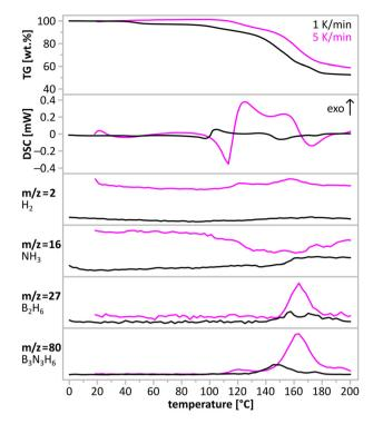
**Fig. 10** Thermogravimetric (TG) and calorimetric (DCS) profiles of the main product set together with MS profiles of the evolved volatile products:  $H_2$  (m/z=2),  $NH_3$  (m/z=16),  $B_2H_6$  (m/z=27), and  $B_3N_3H_6$  (m/z=80). The m/z values were selected among the strongest, noninterfering signals. Scanning rate: 1 K min<sup>-1</sup> (black) and 5 K min<sup>-1</sup> (magenta).
