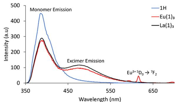
**Fig. 2** Fluorescence spectra of **1H**, **Eu(1)<sub>3</sub>** and **La(1)<sub>3</sub>** showing excimer formation upon complexation (0.01 mM, MeOH,  $\lambda_{\text{ex}} = 300$  nm).
