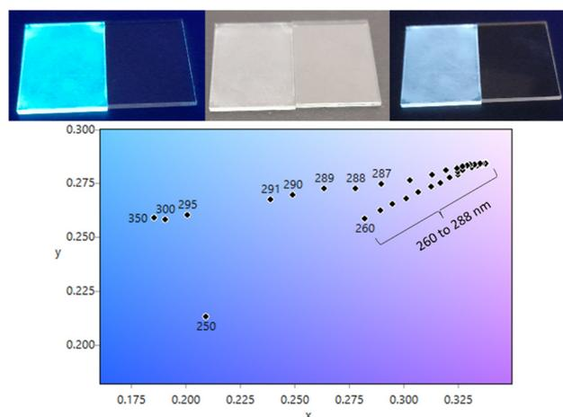
**Fig. 6** (Top) Spin coated films of  $\text{Eu}(\mathbf{1})_3$  on a 15 × 20 mm glass substrate, under 365 nm, ambient light and 254 nm UV irradiation, respectively. (Bottom) CIE coordinates showing the colour-tunable emission range for the  $\text{Eu}(\mathbf{1})_3$  spin coated film (see ESI† for CIE coordinates).
