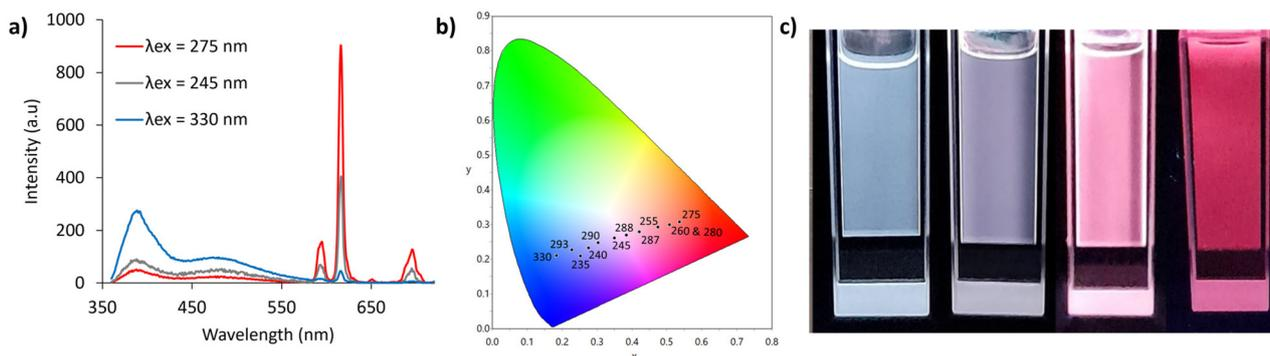
**Fig. 4** (a)  $\text{Eu}(\mathbf{1})_3$  fluorescent emission (0.01 mM, MeOH), showing  $\text{Eu}^{3+}$  centred emission vs. **Nap** centred emission at critical wavelengths. (b) CIE chromaticity diagram showing the colour-tunable emission range of  $\text{Eu}(\mathbf{1})_3$  in solution (0.01 mM, MeOH). (c) Different concentrations of  $\text{Eu}(\mathbf{1})_3$  in MeOH ranging from 10, 5, 1, 0.01 mM left to right, under shortwave UV light ( $\lambda_{\text{ex}} = 254$  nm).
