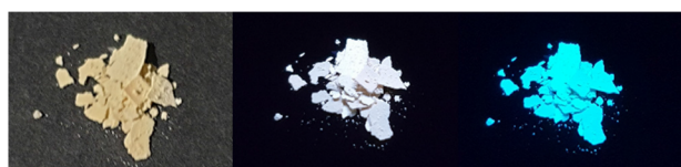
Fig. 5 \text{Eu}(\mathbf{1})_3 solid powder, shown (left to right) under ambient light, 254 nm UV irradiation and 365 nm UV irradiation.
