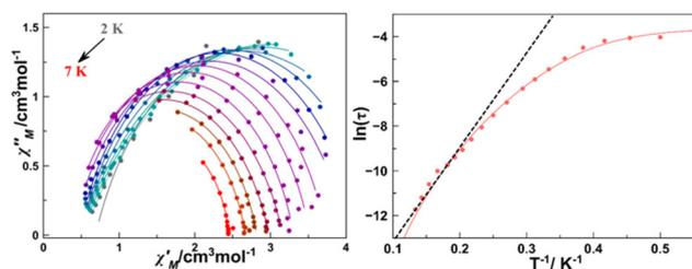
Fig. 6 Left, Argand plot of the magnetic susceptibility of **6**. Right, temperature dependence of the relaxation time as a function of the temperature plotted as  $\ln(\tau)$  vs. inverse of  $T$ . Solid lines show the best fit of the experimental data (Orbach plus Raman fitting) and dotted lines show the slope of the Orbach high temperature regime.
