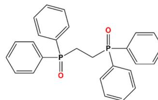
**Scheme 1** Structural formula of the ligand employed in this work, 1,2-bis(diphenylphosphino)ethane dioxide (dppeO<sub>2</sub>).
