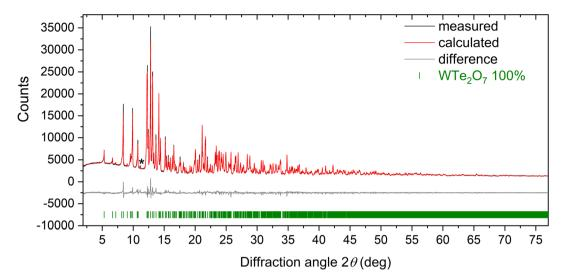
Fig. 5 X-ray powder diffraction pattern (Mo- $K_{\alpha 1}$  radiation) of WTe<sub>2</sub>O<sub>7</sub> and Rietveld refinement (measured (black) and calculated (red) patterns). The calculated reflection positions are indicated by the vertical green bars below the difference pattern ( $R_{\rm exp} = 1.94\%$ ,  $R_{\rm wp} = 3.98\%$ ,  $R_{\rm p} = 3.03\%$ , GooF = 2.05). A small unknown side phase is indicated by an asterisk.
