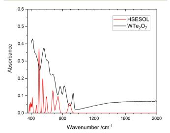
Fig. 9 Comparison of calculated and experimental IR spectrum of WTe<sub>2</sub>O<sub>7</sub>. The theoretical data are based on the HSESOL functional. A shift of the calculated data towards lower energies is visible.
