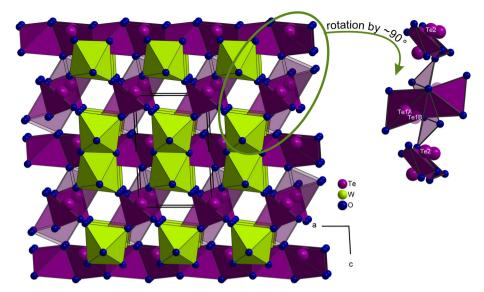
Fig. 3 Crystal structure of WTe<sub>2</sub>O<sub>7</sub> with view along the b-axis.  $[W_2O_{10}]^{8-}$  dimers as well as zweier edge-sharing chains of Te2 atoms running along a are depicted. By increased transparency, the disorder of the Te1 atoms is highlighted and leads to a z-shaped linkage of the chains. On the right side, a structural detail of this linkage is shown.
