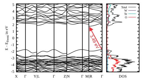
Fig. 7 Band structure and density of states (right part of the figure) of WTe<sub>2</sub>O<sub>7</sub> determined at the HSESOL/double-zeta level.
