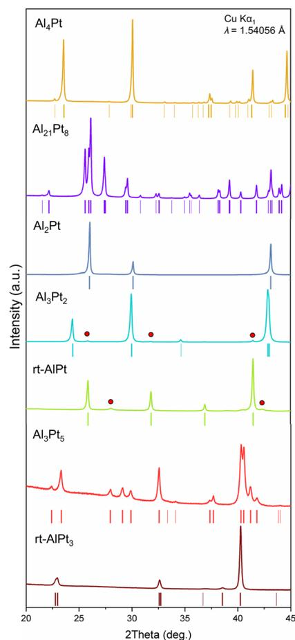
**Fig. 2** PXRD patterns of the prepared Al–Pt compounds. The peak positions of the calculated patterns are shown below the corresponding experimental patterns with colored ticks. The reflections of the secondary phases are marked by red circles.
