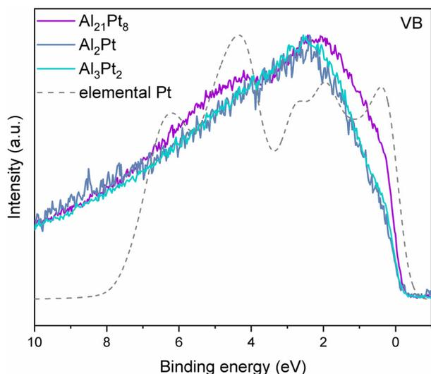
**Fig. 6** Normalized XPS spectra of the valence bands for  $\text{Al}_{21}\text{Pt}_8$ ,  $\text{Al}_2\text{Pt}$  and  $\text{Al}_3\text{Pt}_2$  after 2 h of CP. The grey dashed line represents the calculated sum of the partial DOS for Pt, weighted by photoionization cross-section and broadened by a Gaussian of a full width at half maximum equal to 0.4 eV.
