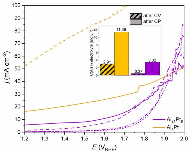
**Fig. 3** LSVs with Al-rich compounds as anode materials: initial (solid lines), after the CV pre-treatment (dashed lines), after one hour of CP (dash-dot lines), and after two hours of CP (short-dash lines). Inset: Concentration of Al in the electrolyte (in  $\text{mg L}^{-1}$ ) after the CV and CP experiments.
