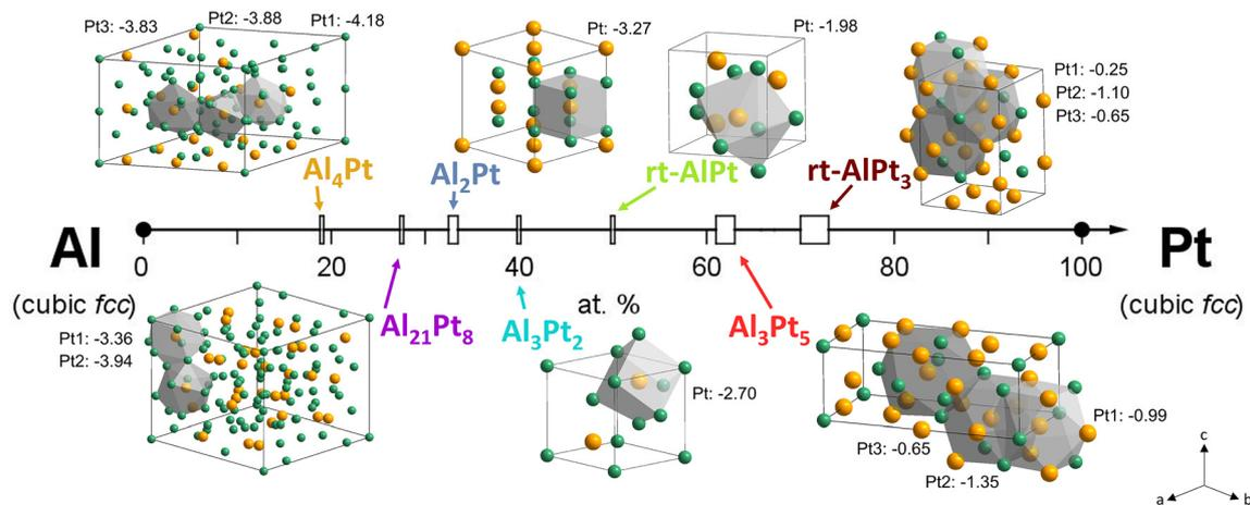
**Fig. 1** Intermetallic Al–Pt compounds and their crystal structures (Pt atoms are in orange and Al in green). The coordination polyhedra are presented for the Pt1, Pt2 and Pt3 atoms. The QTAIM charges of the Pt atoms in the Al–Pt compounds are added from ref. 8.
