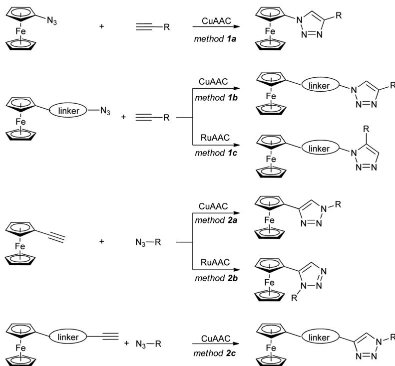
**Scheme 1** General synthetic approaches for ferrocene-1H-1,2,3-triazole conjugates of biological interest. CuAAC – copper catalysed azide–alkyne cycloaddition. RuAAC – ruthenium catalysed azide–alkyne cycloaddition.
