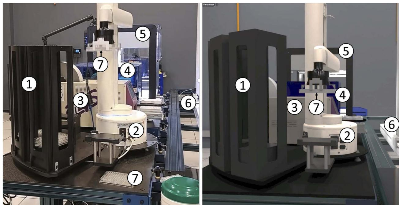
Fig. 10 Other views of the RPL workcell of Fig. 8, shown in real (left) and virtual (right) representations. Modules, from front to back: (1) plate stack; (2) sciclops stacker; (3) a4s\_sealer; (4) brooks\_peeler; (5) ot2; and (6) pf400. Also visible are (7) 96-well plates: one held by the sciclops in each image, and a second on the table in the real case.
