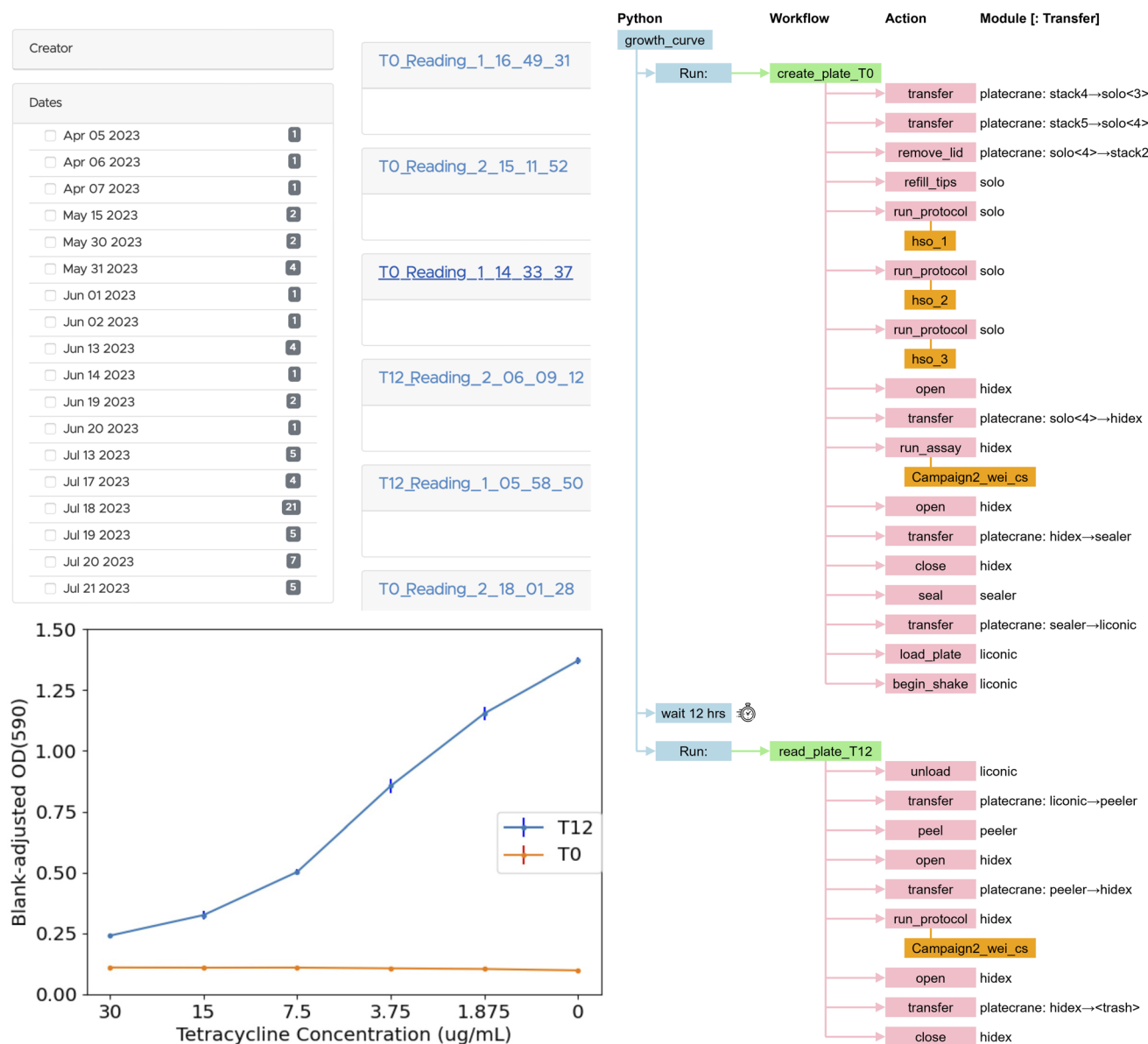
Fig. 15 Growth assay application. Upper left: A list of datasets, one per experiment, on data portal. Lower left: Results from a single experiment in which tetracycline solution at varying concentrations was added to E. coli . Y-axis gives blank-adjusted optical density at 590 nm at the start of the experiment (T0) and 12 hours after start (T12). Results show mean plus error bars from four identical runs. Right: The application, without data analysis and publication steps.
