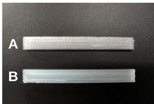
Fig. 5 Examples of impact test samples with different qualities: under-extruded (A) and close to the ideal weight (B).
