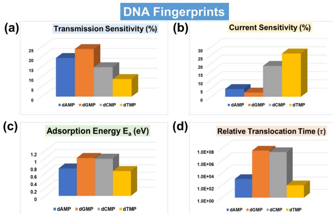
Fig. 7 DNA fingerprints of the AI-integrated MoS<sub>2</sub> nanochannel device. (a) Transmission sensitivity fingerprints of DNA nucleotides at an energy value of 0.635 eV, (b) current sensitivity fingerprints of DNA nucleotides at an applied bias of 0.3 V, (c) adsorption energy fingerprints of DNA nucleotides, and (d) translocation time fingerprints of DNA nucleotides.
