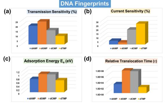
Fig. 7 DNA fingerprints of the Al-integrated  $MoS_2$  nanochannel device. (a) Transmission sensitivity fingerprints of DNA nucleotides at an energy value of 0.635 eV, (b) current sensitivity fingerprints of DNA nucleotides at an applied bias of 0.3 V, (c) adsorption energy fingerprints of DNA nucleotides, and (d) translocation time fingerprints of DNA nucleotides.
