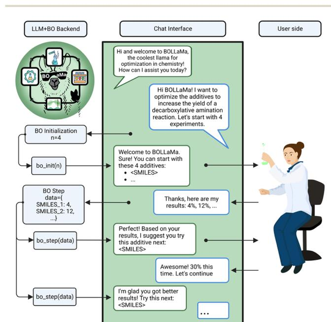
Fig. 6 Schematic overview of BoLLama. An LLM can act as an interface to a BO algorithm. An experimental chemist can bootstrap an optimization and then, *via* a chat interface, update the state of the simulation to which the bot responds with the recommended next steps.
