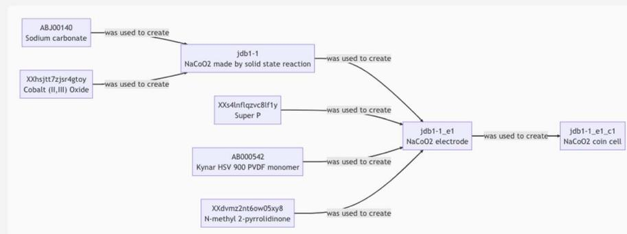
In this flowchart, each rectangular box represents an item in the database, and the arrows between the boxes represent the relationships between the items. For example, SM1 and SM2 were used to create sample JDB1-1, which was then used to create sample E1, which was finally used to create the cell C1.
