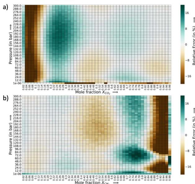
**Fig. 4** Relative error heat maps at the 90% PAC cut-off for  $\text{CO}_2$ - $\text{CH}_4$  mixture, (a)  $\text{CO}_2$  and (b)  $\text{CH}_4$ . The region of  $X_{\text{CO}_2} = 0.02$  to  $0.30$  ( $X_{\text{CH}_4} = 0.70$  to  $0.98$ ) have the highest errors. The model under-predicts adsorption of  $\text{CO}_2$  at  $X_{\text{CO}_2} = 0.02$  to  $0.14$ , and then over-predicts from  $0.14$  to  $0.30$ .
