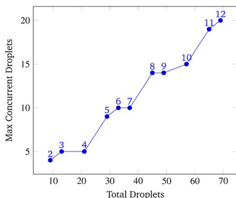
Fig. 17 Max Concurrent droplets vs. total droplets. This data was obtained by running the simulation at a constant grid size of  $45 \times 45$  over a range of gene lengths two to twelve. The number above each point represents the gene length. The vertical axis displays the maximum number of droplets recorded on the chip during the entirety of the simulation while the horizontal axis displays the total amount of droplets pulled from reservoirs to synthesize the gene.
