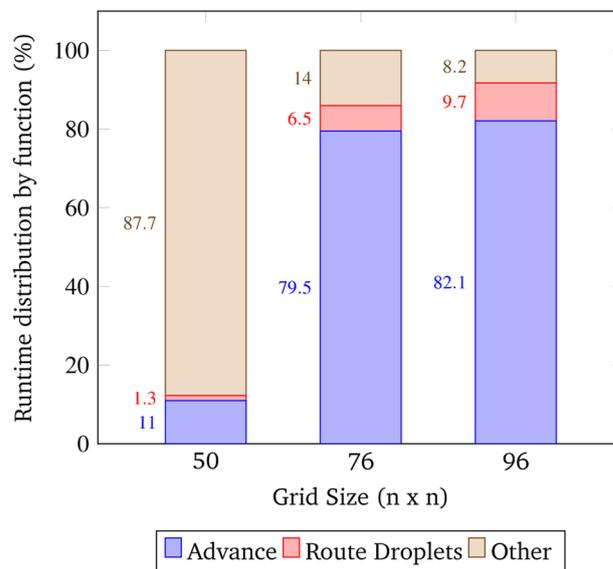
**Fig. 16** Runtime distribution by major function. This data was obtained by running the simulation at an approximately constant congestion ratio. Here the congestion ratio is the total number of droplets pulled from reservoirs divided by the number of grid points. The approximate constant congestion ratio used was 0.0036 droplets gridsizes<sup>-2</sup> which was chosen by convenience. The parameters for these trials are shown in 2.
