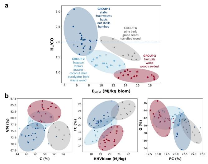
Fig. 5 K-Means cluster analysis based on the gasification outputs. Gasification operating conditions: T = 1173 K, SA = 2.33, and SR = 0.25. (a) Biomass groups identified by the cluster analysis are plotted as a function of the  $E_{vield}$  and  $H_2/CO$  ratio values. (b) Biomass groups identified by the cluster analysis are represented as a function of different biomass properties.
