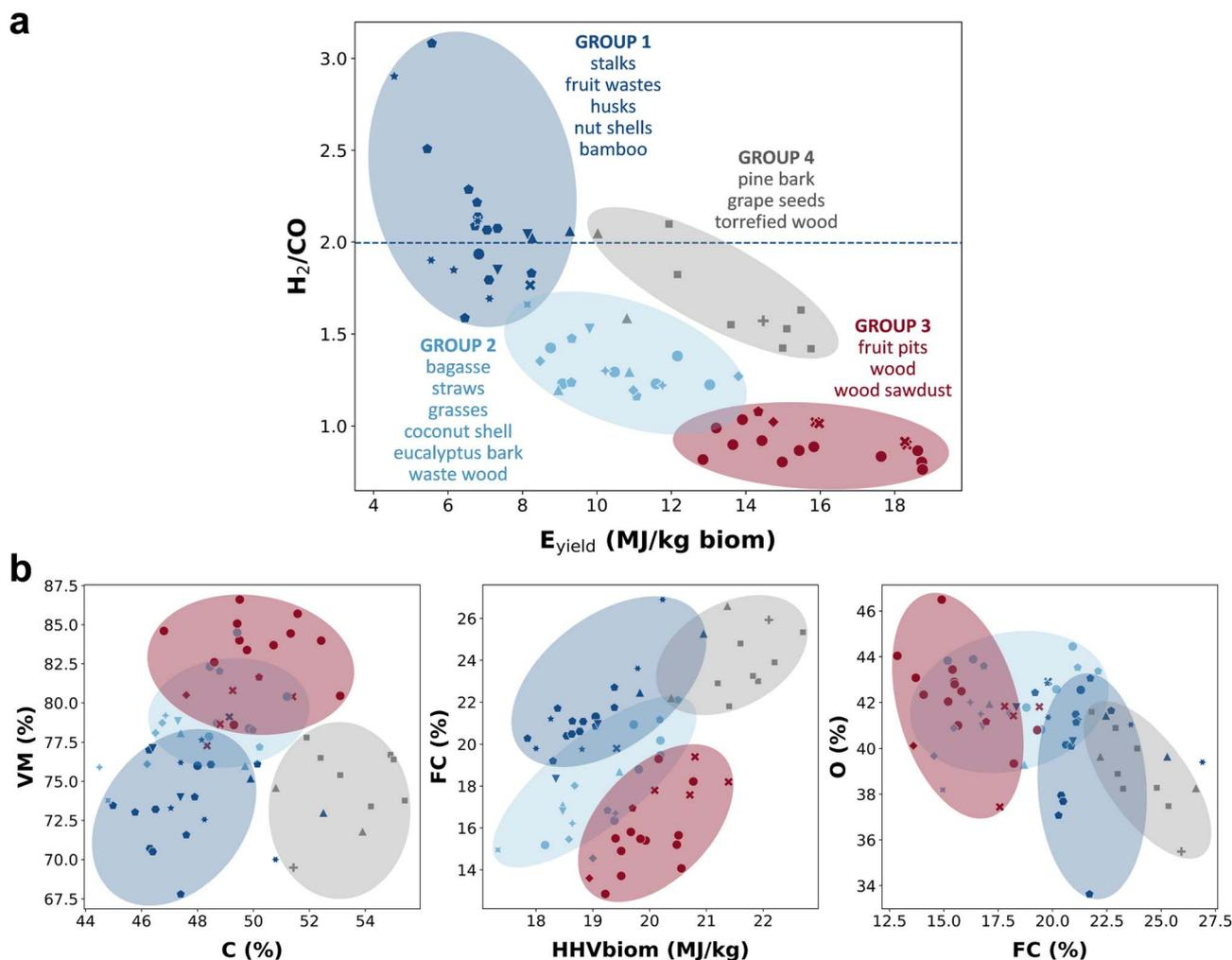
Fig. 5 K-Means cluster analysis based on the gasification outputs. Gasification operating conditions:  $T = 1173$  K,  $SA = 2.33$ , and  $SR = 0.25$ . (a) Biomass groups identified by the cluster analysis are plotted as a function of the  $E_{yield}$  and  $H_2/CO$  ratio values. (b) Biomass groups identified by the cluster analysis are represented as a function of different biomass properties.
