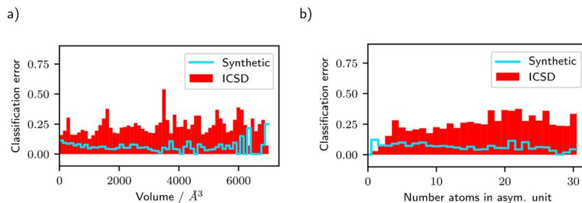
**Fig. 6** Classification error for each bin of (a) the unit cell volume (conventional cell settings) and (b) the number of atoms in the asymmetric unit. The reported classification performance is based on the ResNet-101 model trained on diffractograms from synthetic crystals. This visualization clearly shows the error rate within each bin, in contrast to Fig. 4, which additionally includes the relative proportion of the crystals of the respective bin to the total amount of crystals.
