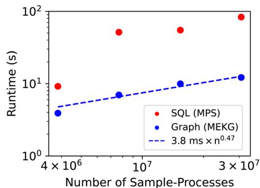
**Fig. 2** Using query 3 from Table 1, the query times for the graph-based query (MekG) and SQL-based query (MPS) are shown using each full database as well as 3 sub-databases with 1/8, 1/4, and 1/2 of the Sample-Processes. The dashed line shows the scaling law from the graph-based query determined *via* linear regression of the log-scaled data points, where  $n$  is the number of Sample-Processes.
