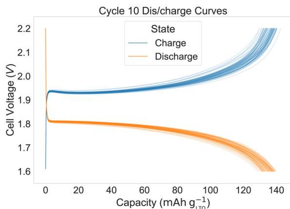
Fig. 3 Charge and discharge curves for cycle 10 of the 80  $\text{LiFePO}_4\|\text{Li}_4\text{Ti}_5\text{O}_{12}$  full cells with dimethyl sulfoxide electrolyte at  $C/2$  rate ( $1C = 150 \text{ mA g}^{-1}$ ). The denser the lines, the bolder the color.
