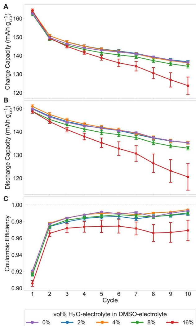
Fig. 5 Specific capacity and energy trends with different volume percent of H<sub>2</sub>O-electrolyte in dimethyl sulfoxide (DMSO)-electrolyte. Error bars are standard error. (A and B) Charge and discharge specific capacity normalized to the mean anode active material (lithium titanate, LTO) vs. cycle. (C) coulombic efficiency computed from (A) and (B) vs. cycle.
