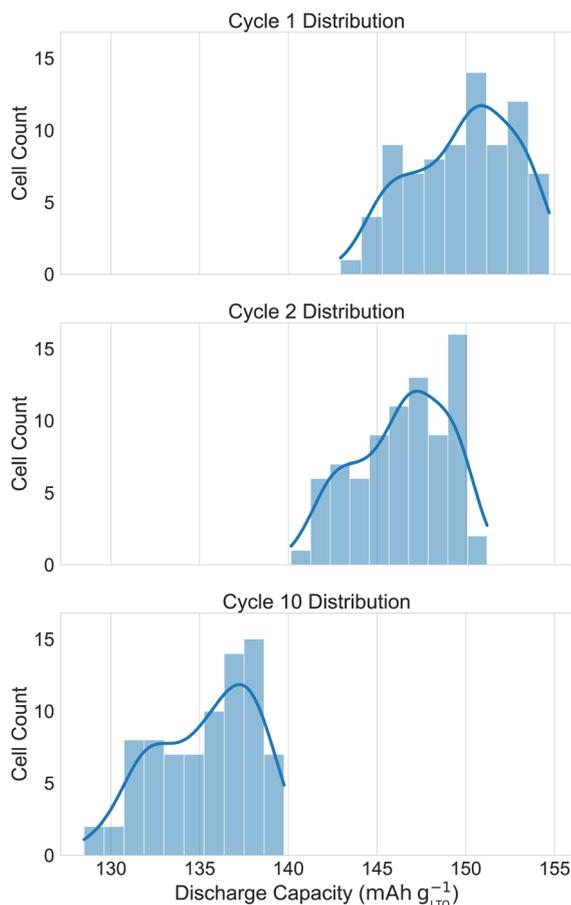
Fig. 2 Distribution of the discharge capacities for the 80 coin cells assembled by the automated robotic setup for cycle 1, 2, and 10. The mean and standard error for cycles 1, 2, and 10 are  $149.8 \pm 0.3 \text{ mA h g}^{-1}$ ,  $146.4 \pm 0.3 \text{ mA h g}^{-1}$ , and  $135.3 \pm 0.3 \text{ mA h g}^{-1}$ , respectively.
