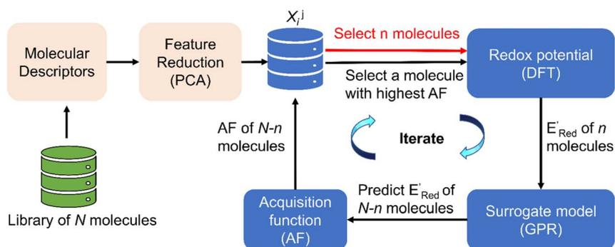
Fig. 2 The AL algorithm to discover promising redoxmers with optimal redox potential in a library of  $N$  molecules. AF is the acquisition function (eqn (6)), DFT is the density functional theory calculations, PCA is the principal component analysis, and GPR is the Gaussian process regression.  $X_i^j$  are the reduced features (principal components with the index  $i$ ) associated with a molecule with the index  $j$ .
