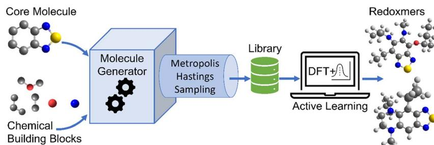
**Scheme 1** Discovery of promising molecules using a Bayesian optimization-based active learning (AL) algorithm and quantum chemistry DFT calculations. The scaffolds and building blocks are combined by molecule generator complemented with a Metropolis type sampler that biases the process to simpler molecules. AL is then used to identify the promising molecules with the minimum DFT calculations.
