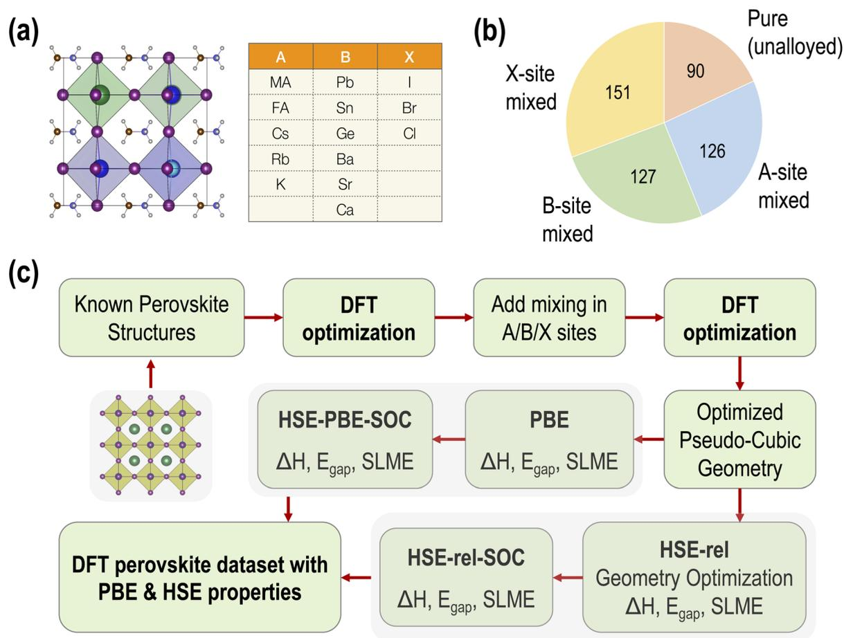
Fig. 1 (a) Chemical space of  $ABX_3$  perovskites studied in this work. (b) Number of samples representing each kind of primary alloy. (c) Steps involved in generating the PBE and HSE datasets of three kinds of properties, namely the decomposition energy ( $\Delta H$ ), band gap ( $E_{\text{gap}}$ ), and spectroscopic limited maximum efficiency (SLME).
