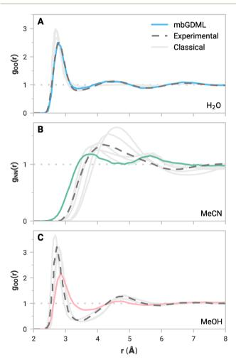
Fig. 3 Simulated RDF curves from NVT MD simulations with mbGDML for (A)  $g_{OO}(r)$  in water, (B)  $g_{NN}(r)$  in acetonitrile, and (C)  $g_{OO}(r)$  in methanol. Reference RDF curves from the literature are shown in dashed gray lines. Examples of classical results in the literature are shown in solid, light gray lines
