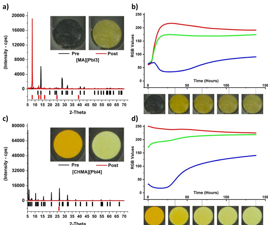
Fig. 4 (a) and (b) Pre/post powder XRD patterns and color change time-series for MAPbI<sub>3</sub>, and (c) and (d) [CHMA][PbI<sub>4</sub>] bulk samples.
