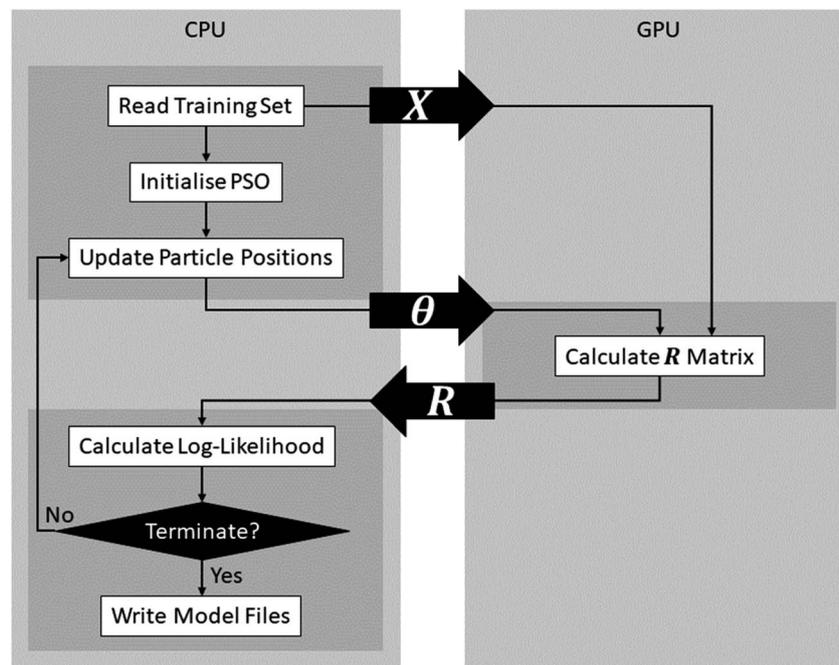
Fig. 10 Details of GPU implementation in FEREBUS.
