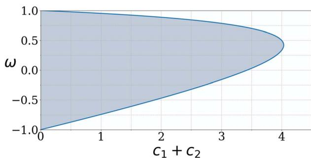
Fig. 3 The shaded section (grey) represents the region of phase space in which the PSO parameters will exhibit convergent behaviour.
