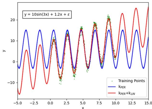
Fig. 1 Demonstration of the effect of combining a periodic and a linear kernel in order to better describe the original function (all plotted with matplotlib).
