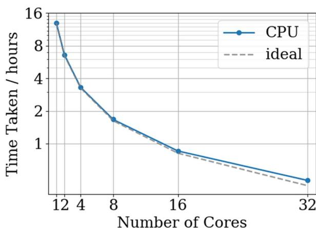
Fig. 9 CPU FEREBUS benchmarks for a 2130-point, 51-dimensional training set running for 1000 PSO iterations with the ideal scaling based upon the serial time.
