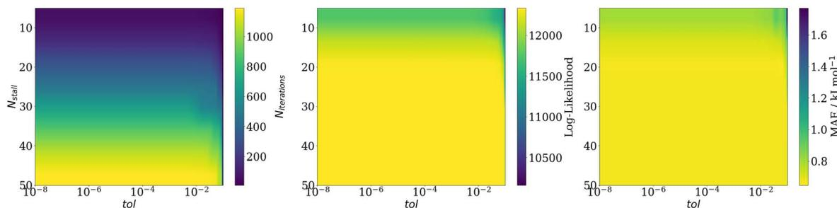
Fig. 6 The effect of the number of stall iterations ( $N_{\text{stall}}$ ) and the tolerance (tol) of the relative difference method on (left) the number of iterations taken to converge, on (middle) the value of the marginal log-likelihood achieved, and on (right) the mean absolute error (MAE) of the resultant model. A 1230-point, 51-dimensional training set was used during the optimisation.
