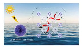
2D photosensitive porphyrin-based MOFs integrated with a Pd cocatalyst with fast charge transfer for efficient photocatalytic hydrogen evolution
