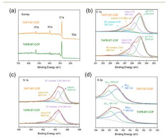
Fig. 2 XPS spectra of the TAPT-BT-COF and TAPB-BT-COF: (a) survey; (b) C 1s; (c) N 1s; and (d) S 2p.
