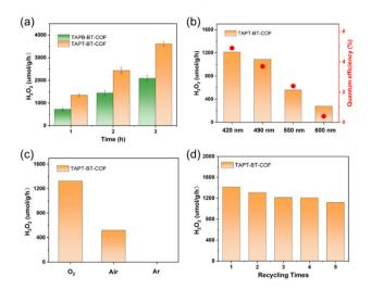
Fig. 5 (a)  $H_2O_2$  production by the two COFs during three hours of reaction. (b) The  $H_2O_2$  production rate and the apparent quantum yield (AQY) of TAPT-BT-COF under different wavelengths (c) and different atmospheres. (d) Recycling of TAPT-BT-COF for 5 cycles.
