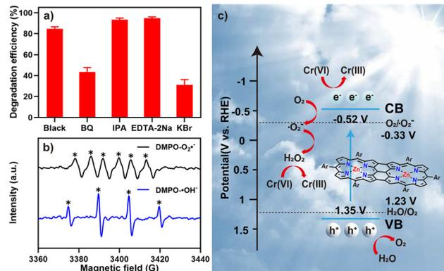
Fig. 5 (a) Photocatalytic reduction of Cr(VI) using **Oligo-Zn-Por** under sunlight irradiation in the presence of different trapping agents (**Oligo-Zn-Por** dosage of 5 mg, trapping agent dosage of 2 mM, Cr(VI) concentration of 70 mg L<sup>-1</sup>); (b) electron spin resonance (ESR) spectra of superoxide radicals and hydroxyl radicals after visible light irradiation for 180 s; (c) sunlight-catalyzed schematic diagram of the **Oligo-Zn-Por** Cr(VI) reduction process.
