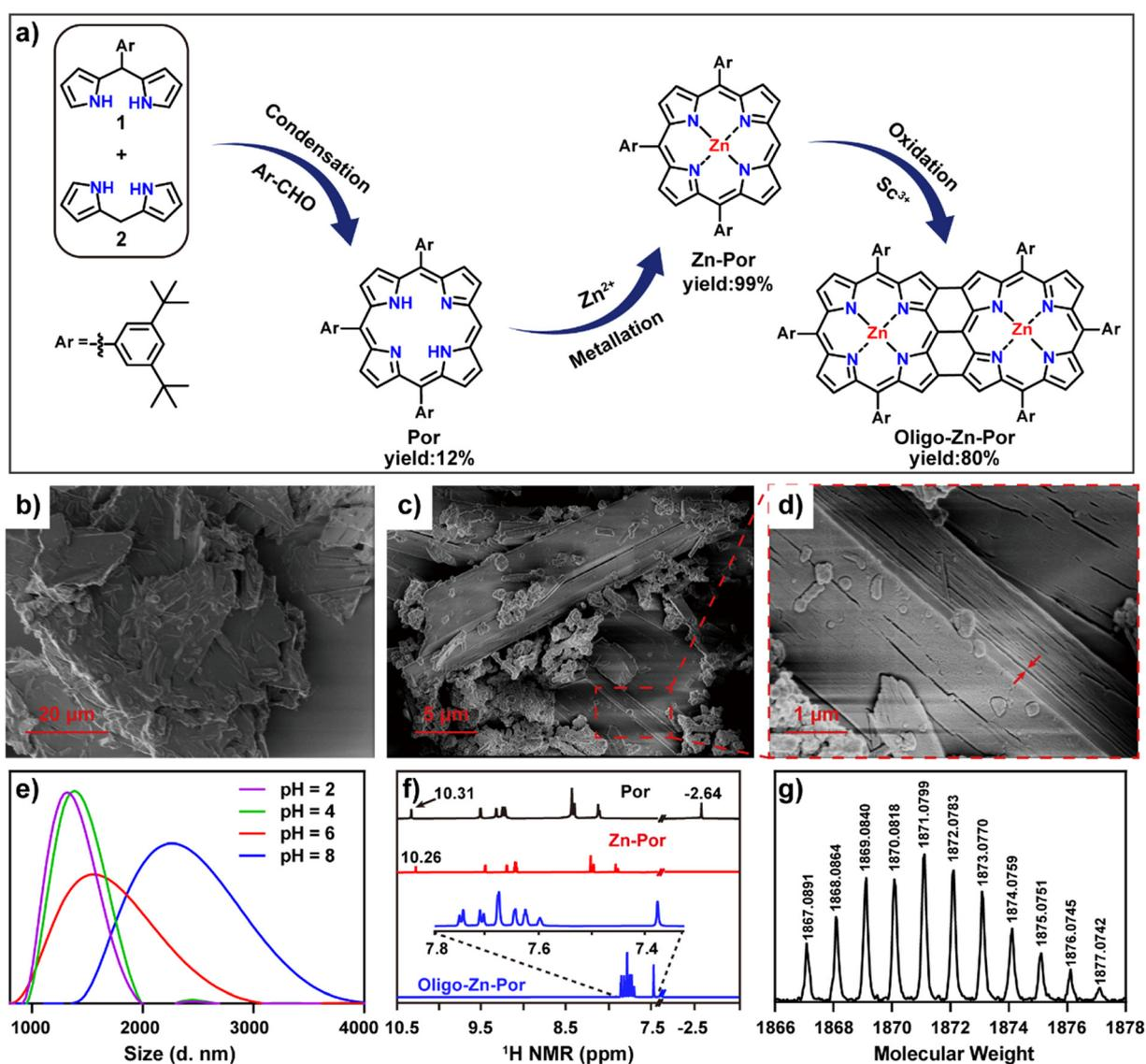
**Fig. 1** (a) Schematic diagram of the **Oligo-Zn-Por** synthetic route and yield; high-resolution field emission scanning electron microscopic images of **Zn-Por** (b) and **Oligo-Zn-Por** (c); (d) magnified view of (c); (e) dynamic light scattering spectra of **Oligo-Zn-Por** at different pH conditions; (f)  $^1\text{H}$  NMR spectra of **Por**, **Zn-Por**, and **Oligo-Zn-Por**; (g) high-resolution mass spectra of **Oligo-Zn-Por**.
