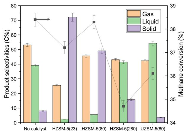
**Fig. 2** The methane conversion and product selectivities of UZSM-5, and HZSM-5 catalysts with various SiO<sub>2</sub>/Al<sub>2</sub>O<sub>3</sub> ratios.
