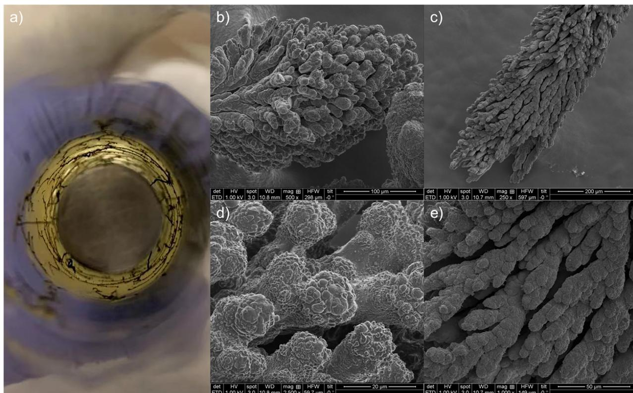
**Fig. 3** Pictures of the coke generated between the electrode and the quartz tube. a) the picture of the spent reactor; b–e) the SEM images of the coke.
