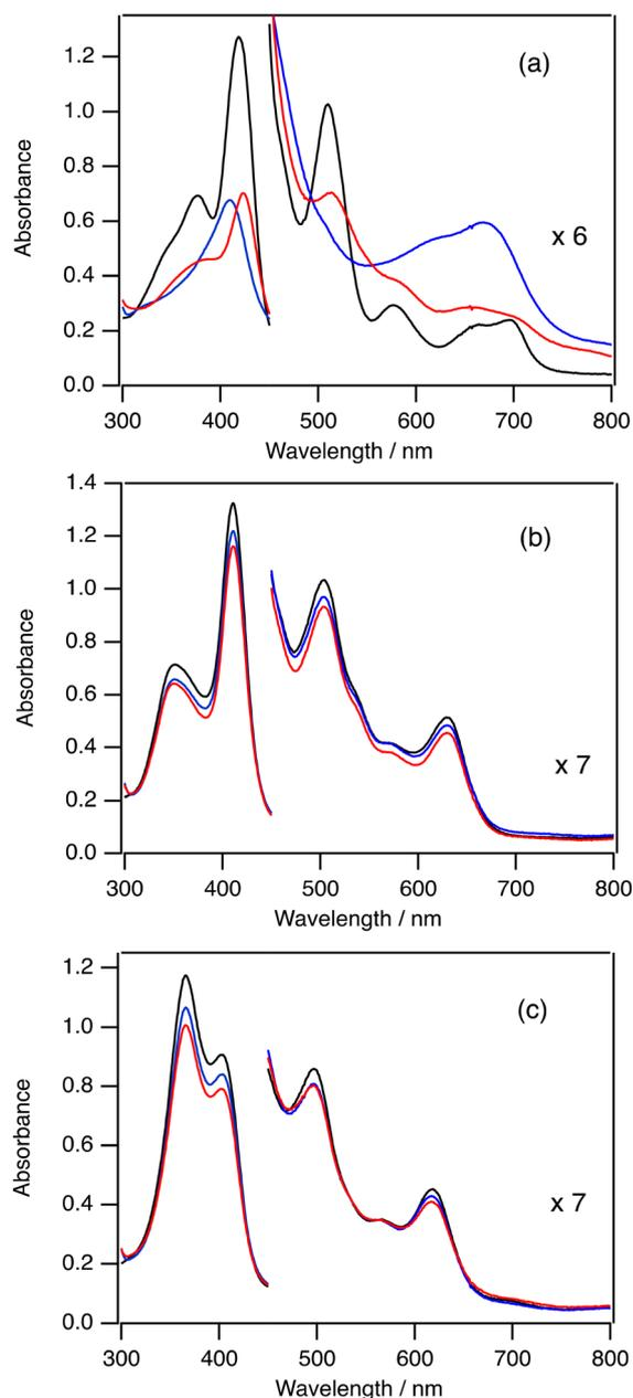
**Fig. 3** Absorption spectral changes in the catalytic cyclohexane oxidation reactions of 2-Cl (a), 3-Cl (b), and 5-Cl (c) with mCPBA at 20 °C. Black line: before addition of mCPBA, blue line: immediately after the addition of mCPBA, red line: after 300 s.
