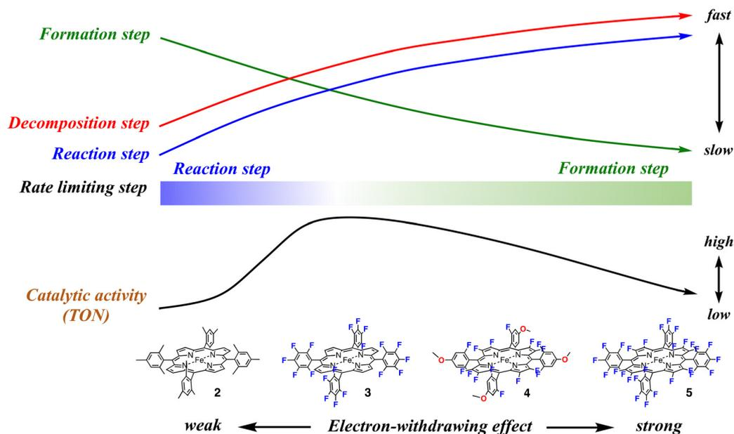
Fig. 7 Electron-withdrawing effect of the porphyrin substituent on the rates of the formation (green arrow), reaction (blue arrow), and decomposition (red arrow) steps, and on the overall catalytic activity (TON) for the cyclohexane oxidation reaction (black arrow). The bar of the rate limiting step indicates the change of the rate limiting step with an increase in the electron-withdrawing effect.
