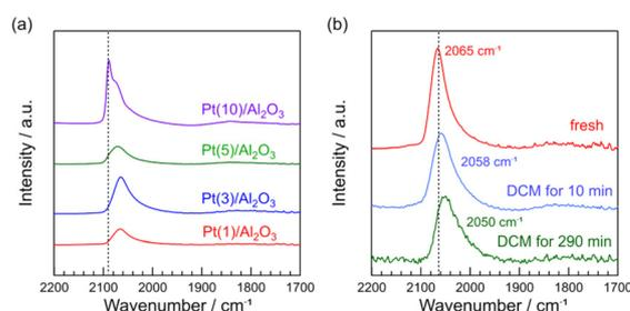
**Fig. 5** FT-IR spectra of chemisorbed CO on Pt/Al<sub>2</sub>O<sub>3</sub> catalysts. (a) fresh Pt(1, 3, 5, and 10)/Al<sub>2</sub>O<sub>3</sub> and (b) fresh and spent Pt(1)/Al<sub>2</sub>O<sub>3</sub>. DCM reaction conditions:  $T = 600$  °C, flow rate =  $20 + 1$  (CH<sub>4</sub> + H<sub>2</sub>) mL min<sup>-1</sup>, catalyst mass = 0.10 g.
