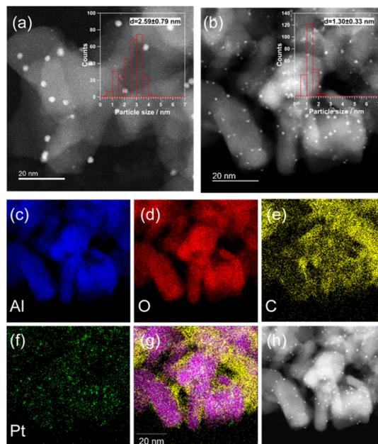
Fig. 2 HAADF-STEM images and particle size distribution of (a) fresh and (b) spent  $\text{Pt}(1)/\text{Al}_2\text{O}_3$ . EDX mapping images for (c) Al, (d) O, (e) C, (f) Pt, (g) overlay of (c-f), and (h) HAADF-STEM image of the spent catalyst. Spent catalyst: DCM was performed on  $\text{Pt}(1)/\text{Al}_2\text{O}_3$  for 5 h under  $\text{CH}_4/\text{H}_2$  (20/1).
