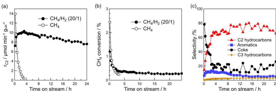
Fig. 6 Time course of (a) formation rate of C<sub>2</sub> hydrocarbons, (b) methane conversion, and (c) product selectivity for DCM reaction. Catalyst: Pt(1)/Al<sub>2</sub>O<sub>3</sub>, T: 600 °C, flow rate: 20 (CH<sub>4</sub>) and 20 + 1 (CH<sub>4</sub> + H<sub>2</sub>) mL min<sup>-1</sup>, and catalyst mass: 0.10 g.
