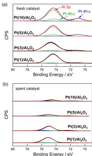
**Fig. 4** Pt 4f and Al 2p XPS of (a) fresh and (b) spent Pt(1, 3, 5, and 10)/Al<sub>2</sub>O<sub>3</sub> catalysts. DCM reaction conditions:  $T = 600$  °C, flow rate =  $20 + 1$  (CH<sub>4</sub> + H<sub>2</sub>) mL min<sup>-1</sup>, and catalyst mass = 0.10 g.
