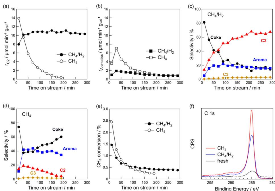
Fig. 1 Time course of formation rate of (a)  $\text{C}_2$  hydrocarbons and (b) aromatics, (c and d) product selectivity, and (e)  $\text{CH}_4$  conversion for DCM reaction. (f) C 1s XPS of  $\text{Pt}(1)/\text{Al}_2\text{O}_3$  before and after DCM. Catalyst:  $\text{Pt}(1)/\text{Al}_2\text{O}_3$ ,  $T$ : 600 °C, flow rate: 20 ( $\text{CH}_4$ ) and 20 + 1 ( $\text{CH}_4 + \text{H}_2$ )  $\text{mL min}^{-1}$ , and catalyst mass: 0.10 g.
