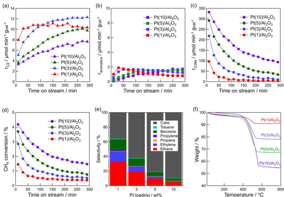
Fig. 3 Time course of formation rate of (a) C<sub>2</sub> hydrocarbons, (b) aromatics, (c) coke, and (d) CH<sub>4</sub> conversion for DCM reaction. (e) Product selectivity for DCM reaction. (f) TG profiles of the spent catalysts. Catalyst: Pt(1, 3, 5, and 10)/Al<sub>2</sub>O<sub>3</sub>, T: 600 °C, flow rate: 20 + 1 (CH<sub>4</sub> + H<sub>2</sub>) mL min<sup>-1</sup>, and catalyst mass: 0.10 g.
