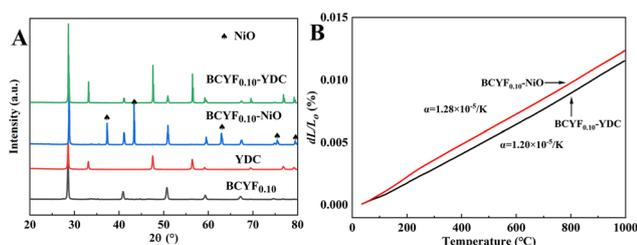
Fig. 4 (A) Powder XRD pattern and (B) thermal expansion curves of BCYF<sub>0.10</sub>-YDC and BCYF<sub>0.10</sub>-NiO monolayer HF membranes and membrane material powders.
