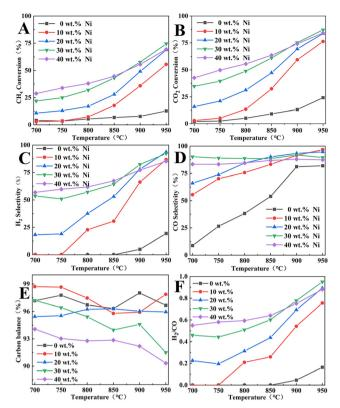
Fig. 10 DRM catalytic performance of Ni/BCYF<sub>0.10</sub>-YDC catalysts with different Ni contents: (A) CH<sub>4</sub> and (B) CO<sub>2</sub> conversion, (C) H<sub>2</sub> and (D) CO selectivity. (E) carbon balance, and (F) H<sub>2</sub>/CO molar ratio (feed gas was 50 mL min<sup>-1</sup> CH<sub>4</sub> and 50 mL min<sup>-1</sup> CO<sub>2</sub>).
