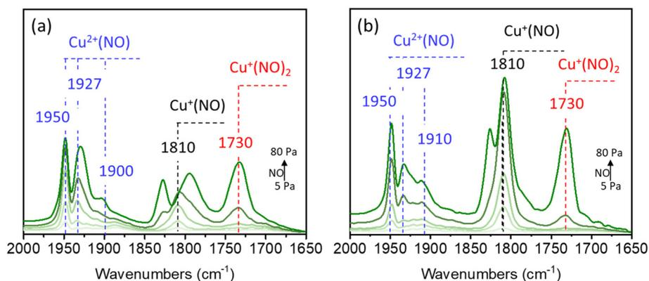
**Fig. 2** NO (5–80 Pa) adsorption FTIR spectra over (a) 5Cu/AEI-C and (b) 5Cu/AEI-S zeolite catalysts collected at  $-120\text{ }^\circ\text{C}$  after pretreatment at  $500\text{ }^\circ\text{C}$  in a vacuum for 1 h.
