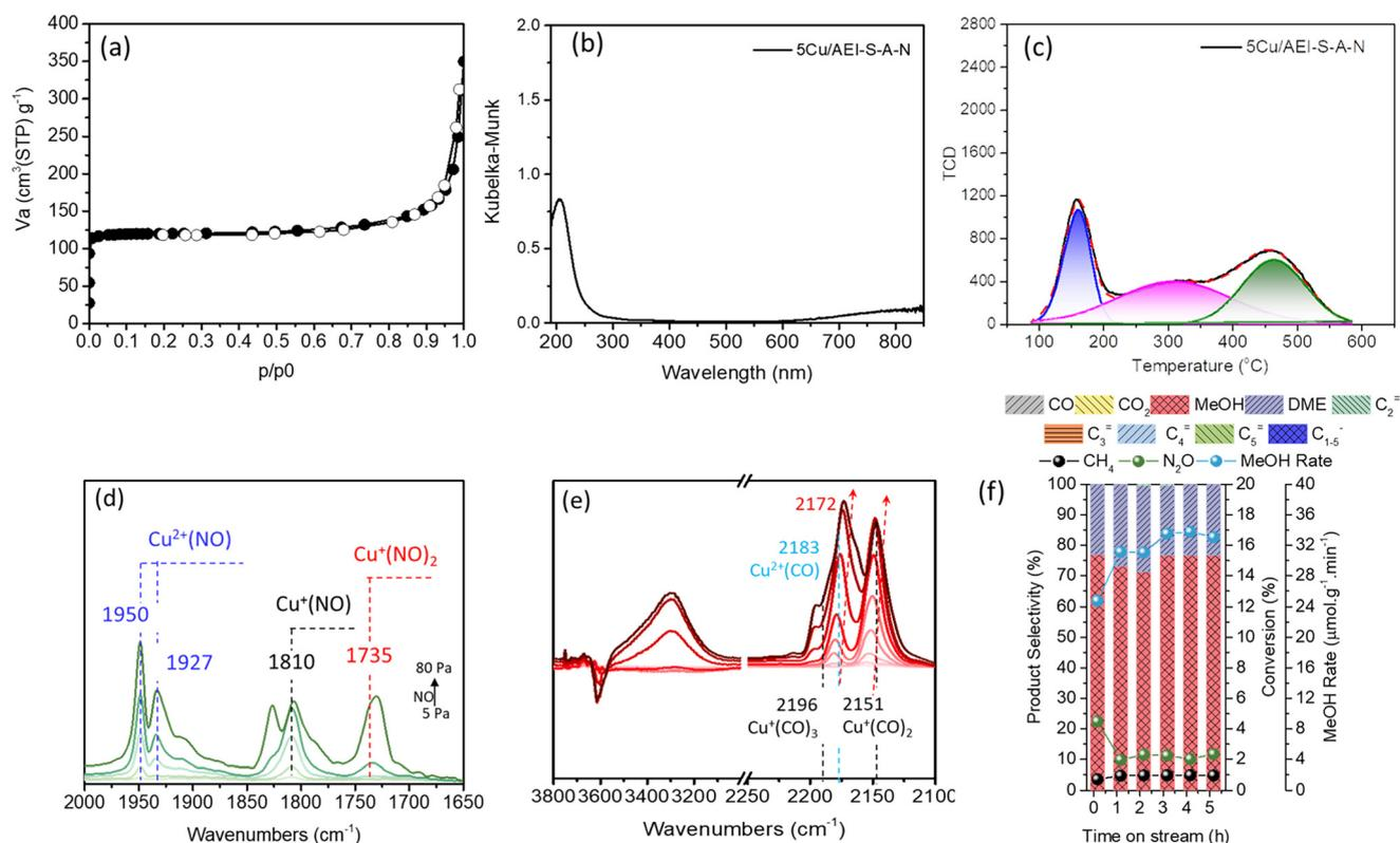
**Fig. 8** (a) N<sub>2</sub> adsorption and desorption isotherms, (b) UV-vis spectrum, (c) NH<sub>3</sub>-TPD curve, (d) NO (5–120 Pa) adsorption FTIR spectrum, and (e) CO (5–1000 Pa) adsorption FTIR spectrum of the 5Cu/AEI-S-A-N zeolite catalyst. (f) Stability test of 100 mg of the 5Cu/AEI-S-A-N zeolite catalyst at 350 °C, CH<sub>4</sub>/N<sub>2</sub>O/H<sub>2</sub>O/Ar = 10/10/2/3 ml min<sup>-1</sup>, SV = 15 000 ml g<sup>-1</sup> h<sup>-1</sup>.
