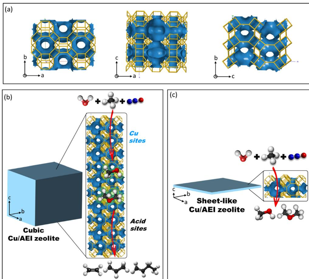
**Scheme 1** (a) Channel systems of AEI zeolite seen from different directions. (b) Schematic view of methanol production from methane and diffusion within the Cu/AEI-C zeolite along the *c*-axis to produce olefins. (c) Schematic view of methanol production from methane and outward diffusion along the *c*-axis of the Cu/AEI-S zeolite.
