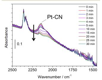
Fig. 7 In situ FTIR spectroscopy results for the reaction of CH<sub>4</sub> and NO followed by He purge and hydrogen treatment on the Pt/Al<sub>2</sub>O<sub>3</sub> catalyst at 425 °C. Time (min) indicates that treated with hydrogen.
