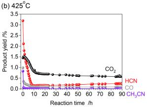
Fig. 2 Time-course of the reaction for methane with nitric oxide over the Pt/Al<sub>2</sub>O<sub>3</sub> catalyst at 400 °C (a) and 425 °C (b). Reaction conditions: 5 wt% Pt/Al<sub>2</sub>O<sub>3</sub> (100 mg), CH<sub>4</sub>: NO: He = 13.4:1.8:84.8 (total flow rate: 100 mL min<sup>-1</sup>), and 0.1 MPa.
