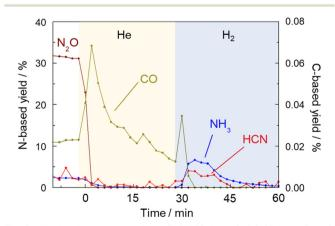
Fig. 8 Yields of gaseous products (HCN (C-based), CO (C-based), N<sub>2</sub>O (N-based), and NH<sub>3</sub> (N-based)) determined by FTIR spectroscopy during the reaction CH<sub>4</sub>-NO (before 0 min), He purging (0-28 min), and H2 treatment (after 28 min).
