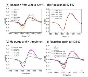
Fig. 6 Pt L<sub>3</sub>-edge XANES difference spectra subtraction of the spectrum just before the introduction of CH<sub>4</sub> and NO mixture. (a) Reaction from 300 to 425  $^{\circ}$ C, (b) reaction at 425  $^{\circ}$ C, (c) He purge and H<sub>2</sub> treatment after the first reaction at 425 °C, (d) the second reaction at 425 °C after He purge and H2 treatment.
