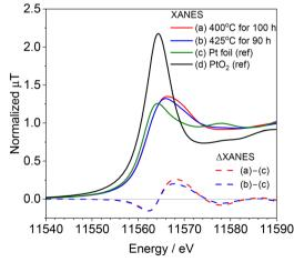
Fig. 3 Pt  $L_3$ -edge XANES spectra of the  $Pt/Al_2O_3$  catalyst after the reaction with methane and nitric oxide at 400 °C for 100 h or 425 °C for 90 h, and the difference XANES spectra of the spent catalysts and Pt foil.
