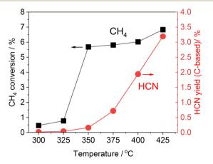
Fig. 1 Methane conversion and hydrogen cyanide yield (carbonbased) as a function of temperature for the reaction of methane with nitric oxide over the Pt/Al<sub>2</sub>O<sub>3</sub> catalyst. Reaction conditions: 5 wt% Pt/  $Al_2O_3$  (100 mg),  $CH_4:NO:He = 13.4:1.8:84.8$  (total flow rate: 100 mL  $min^{-1}$ ), and 0.1 MPa.
