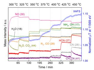
Fig. 4 Changes of the MS spectra and the XAFS intensity (at 11569 eV) at various temperatures raising from 300 to 450 °C with 25 °C steps. Reaction conditions: 5 wt% Pt/Al<sub>2</sub>O<sub>3</sub> (100 mg), CH<sub>4</sub>: NO: He = 13.4: 1.8:84.8 (total flow rate: 100 mL min<sup>-1</sup>), and 0.1 MPa.
