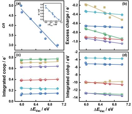
Fig. 2 Relationships between the formation energy of S vacancies ( $\Delta E_{Vac}$ ) on MoS<sub>2</sub>(001) and: (a) the number of S atoms coordinated to Mo atoms (cn). Inset: Correlation between  $\Delta E_{Vac}$  and work function ( $\phi$ ). (b) The excess charge on the adsorbates. (c) Integrated crystal orbital overlap population (coop). (d) Integrated crystal orbital Hamilton population (cohp) upon atom adsorption. The data in this figure are in Tables S1 and S2† (section S9).
