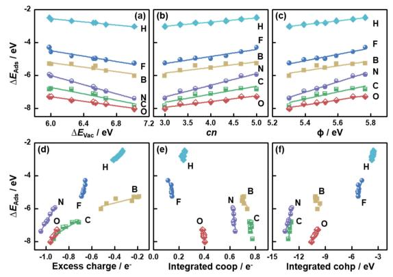
Fig. 4 Adsorption energies ( $\Delta E_{Ads}$ ) of atomic species on MoS<sub>2</sub>(001) as a function of (a) the formation energies of S vacancies ( $\Delta E_{Vac}$ ); (b) the number of S atoms coordinated to Mo atoms (cn); (c) work function (φ); (d) the excess charge on the adsorbates; (e) integrated crystal orbital overlap population (coop); and (f) crystal orbital Hamilton population (cohp). The data in this figure can be found in Tables S3-S9.†
