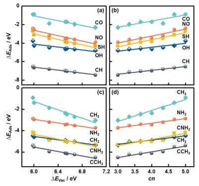
Fig. 5 Adsorption energies ( $\Delta E_{Ads}$ ) of molecules on MoS<sub>2</sub>(001) as a function of (a and c) the formation energies of S vacancies ( $\Delta E_{Vac}$ ), and (b and d) the number of S atoms coordinated to Mo atoms (cn). See the data in this figure in Tables S11-S14.†
