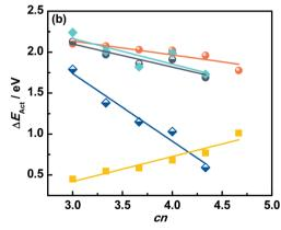
Fig. 6 Reaction energies  $\Delta H$  (a) and activation energies  $\Delta E_{Act}$  (b) of various elementary reactions as a function of the number of S atoms coordinated to Mo atoms (cn) on MoS<sub>2</sub>(001). The slopes for \*NO dissociation are positive because  $\Delta H$  and  $\Delta E_{Act}$  are mostly determined by the products instead of reactants, as opposed to the recombination reactions. The data in this figure appear in Tables S15 and S16.†
