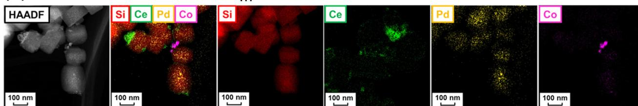
Fig. 23 STEM-EDS images of (A) 1 wt% Pd-1 wt% Co/Ce-MFI<sub>MC</sub> and (B) 1 wt% Pd-1 wt% Co/Ce-MFI<sub>HT</sub>. Reproduced from ref. 88 with permission from American Chemical Society, copyright 2022.
