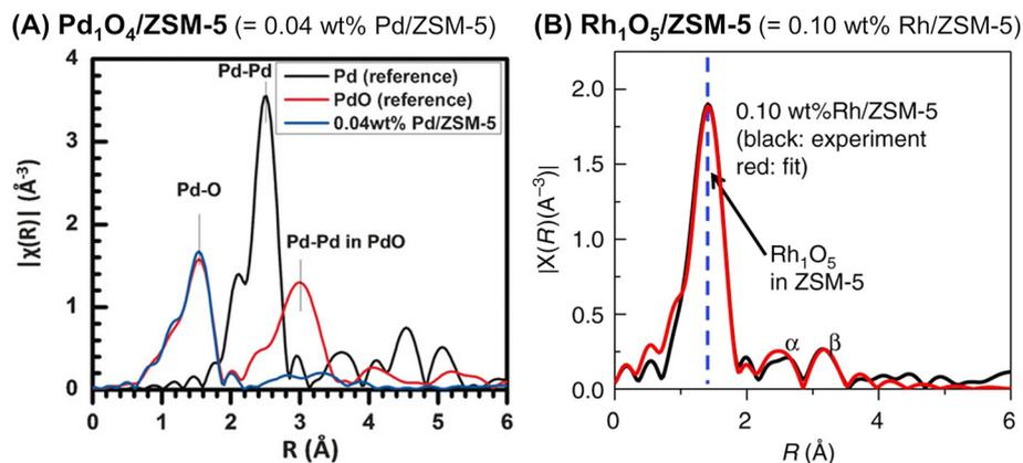
Fig. 21 Fourier transform of EXAFS spectra of (A) Pd<sub>1</sub>O<sub>4</sub>@ZSM-5 ( $k^2$ -weighted Pd K-edge) and (B) Rh<sub>1</sub>O<sub>5</sub>@ZSM-5 ( $k^2$ -weighted Rh K-edge). Reprinted from (A) ref. 81 with permission from John Wiley and Sons, copyright 2016, and (B) ref. 82 with permission from Springer Nature, copyright 2018.
