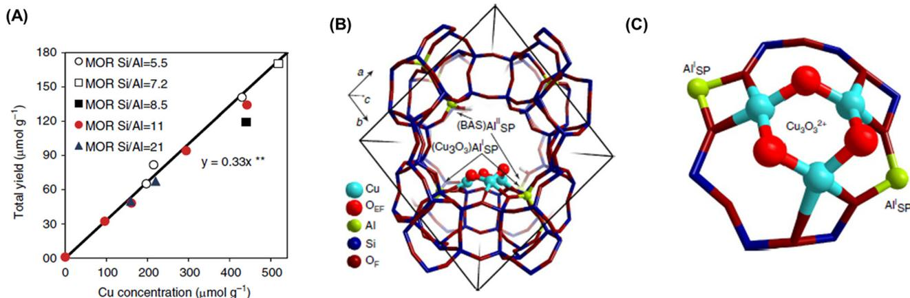
Fig. 9 (A) Total yield of methanol over Cu-MOR with different Si/Al ratios and Cu concentrations. (B) Location and (C) structure of  $[\text{Cu}_3(\mu\text{-O})_3]^{2+}$  cluster in MOR determined by DFT calculations. Reproduced from ref. 47 with permission from Springer Nature, copyright 2015.
