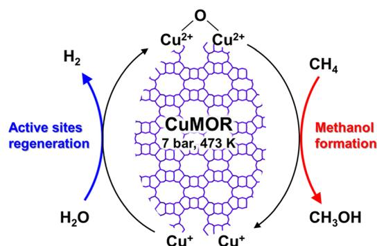
Fig. 10 Plausible reaction scheme for partial oxidation of methane to methanol over Cu-MOR *via* the chemical looping process, using water as an oxidant.
