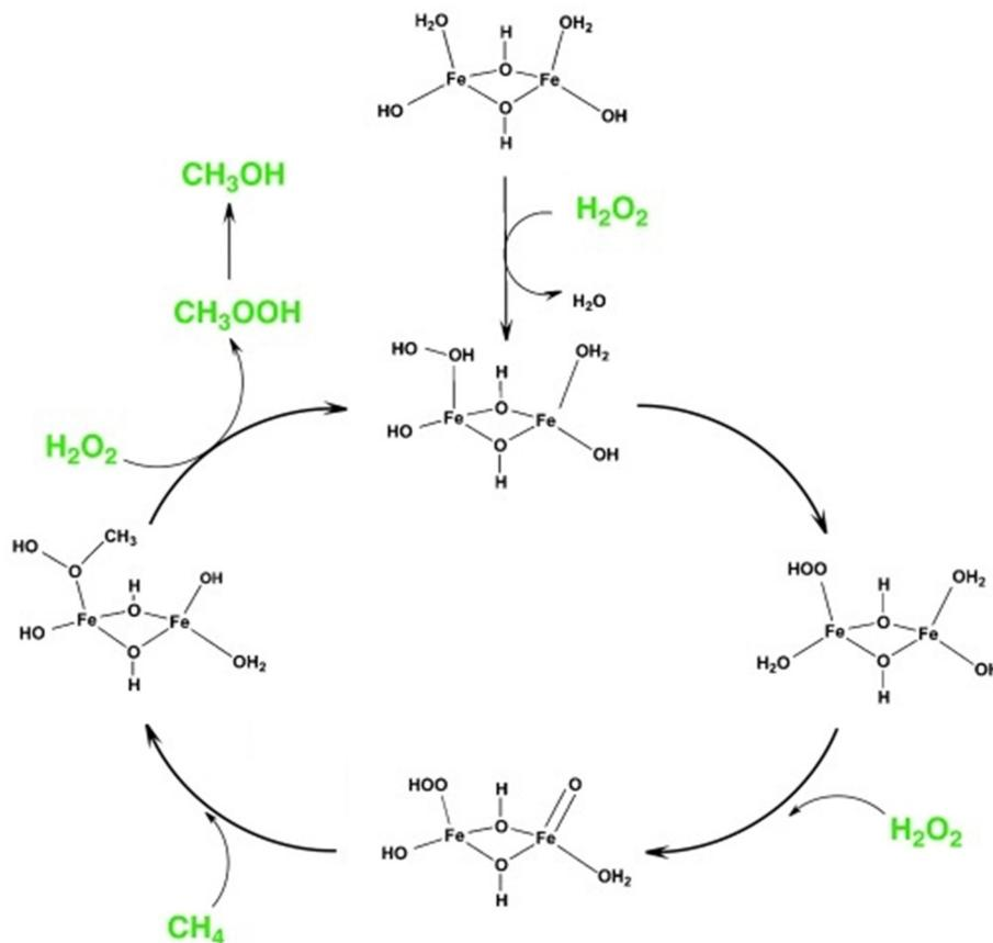
Fig. 5 Proposed reaction mechanism of MTM reaction over the active site of  $[\text{Fe}_2(\mu_2\text{-OH})_2(\text{OH})_2(\text{H}_2\text{O})_2]^{2+}$  in Fe-containing ZSM-5. Reprinted from ref. 30 with permission from John Wiley and Sons, copyright 2012.
