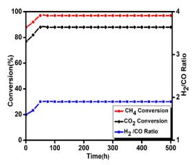
Fig. 8 Effect of time on stream for 5Ni–5Co-mod alumina at 850 °C with WHSV 10 L  $g^{-1}$  h<sup>-1</sup> at atmospheric pressure. Prior to the activity study, the catalyst was reduced at 850 °C with 20% H<sub>2</sub>/N<sub>2</sub>.
